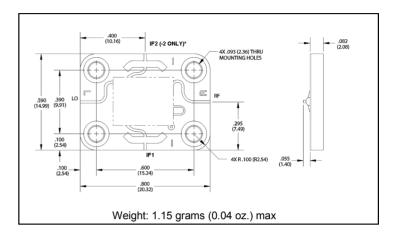
\*For the base model, only IF1 port is connected. For the -"-2" model, only IF2 port is connected.
