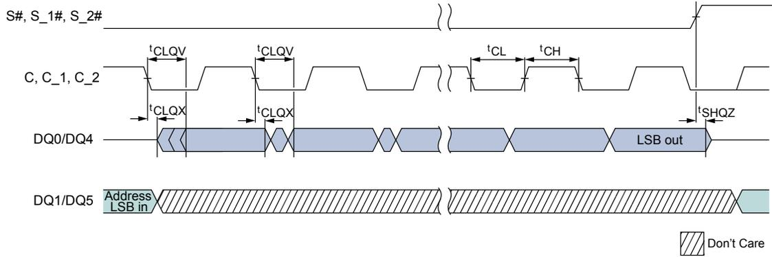
**Figure 56: Output Timing for DTR**
