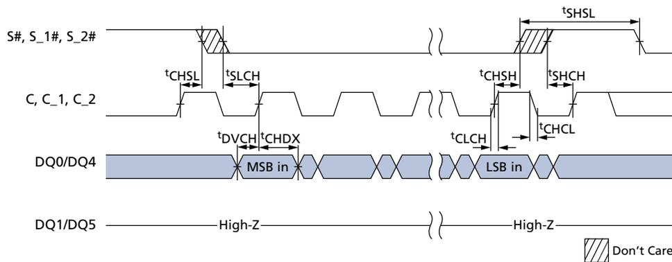
**Figure 52: Serial Input Timing DTR**
