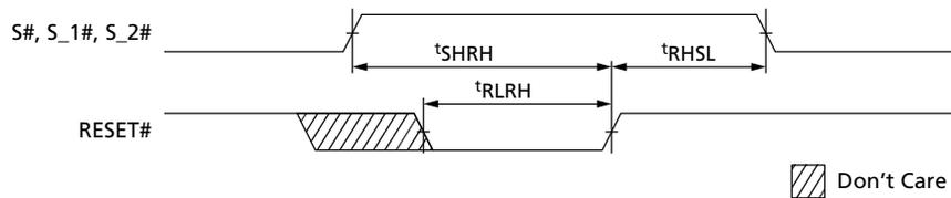
**Figure 50: Reset Enable and Reset Memory Timing**
