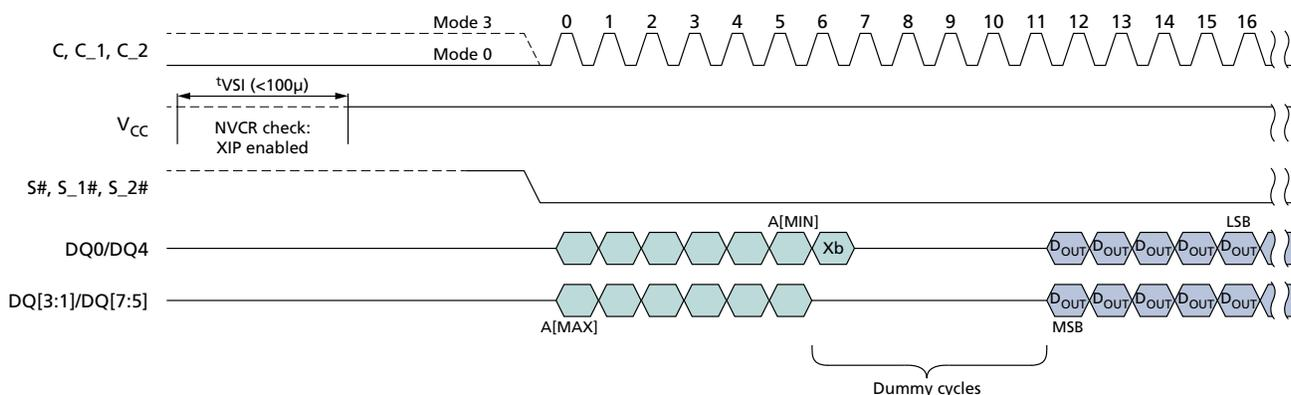
Note: 1. Xb is the XIP confirmation bit and should be set as follows: 0 to keep XIP state; 1 to exit XIP mode and return to standard read mode.
