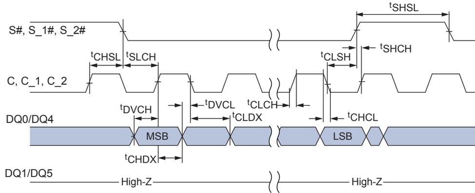
**Figure 53: Write Protect Setup and Hold During WRITE STATUS REGISTER Operation (SRWD = 1)**
