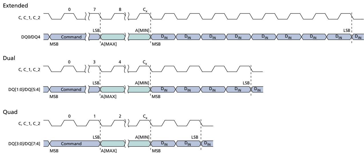
Note: 1. For extended SPI protocol,  $C_x = 7 + (A[MAX] + 1)$ ; For dual SPI protocol,  $C_x = 3 + (A[MAX] + 1)/2$ ; For quad SPI protocol,  $C_x = 1 + (A[MAX] + 1)/4$ .
