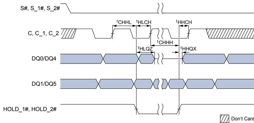
**Figure 55: Output Timing for STR**
