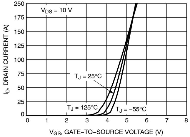
Figure 2. Transfer Characteristics
