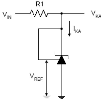
Test Circuit 4 for V<sub>KA</sub> = V<sub>REF</sub>
