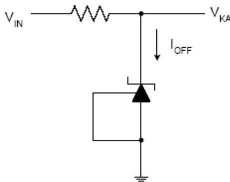
Test Circuit 6 for I<sub>OFF</sub>
