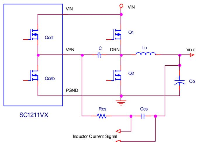
The above circuit shows the concept of Combi-Sense® technique. An internal totem pole (Qcst, Qcsb) generates a VPN (Virtual Phase Node) signal. This VPN follows the DRN (or the Power Phase Node) with the same timing. A RC network (Rcs and Ccs) is connected between
