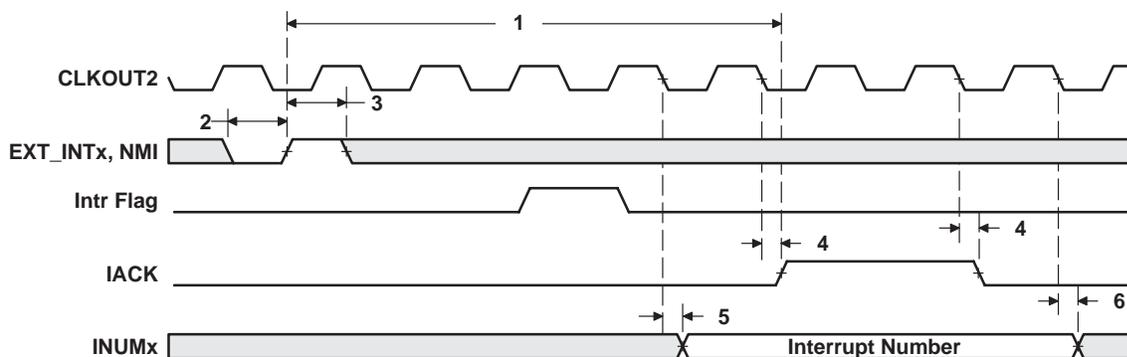
Figure 29. Interrupt Timing
