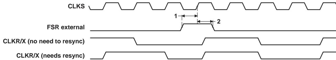
**Figure 34. FSR Timing When GSYNC = 1**
