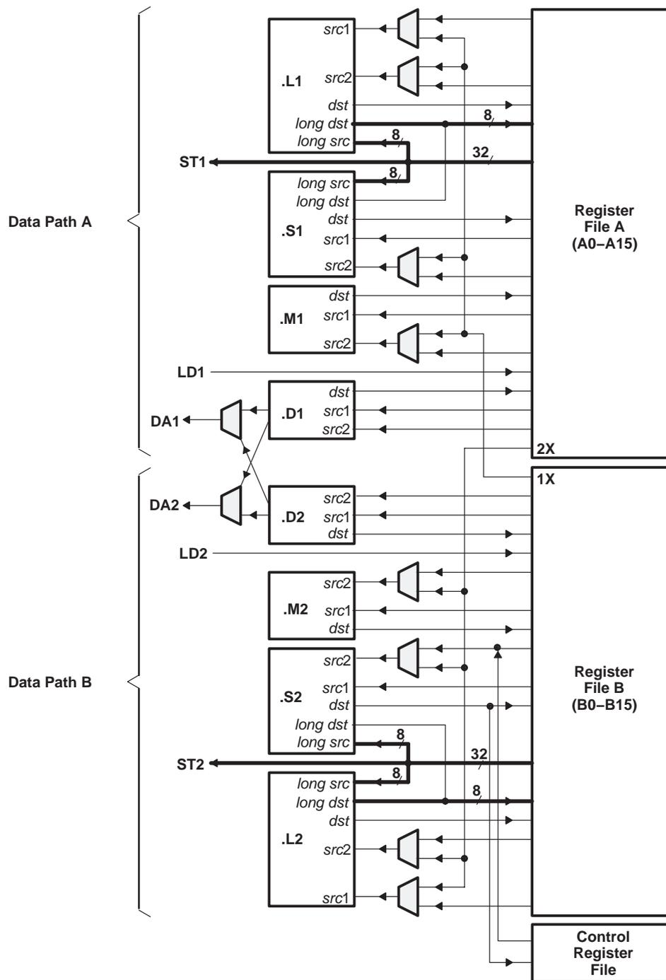
Figure 1. TMS320C62x CPU (DSP Core) Data Paths
