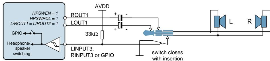
**Figure 21 Example Headset Detection Circuit Using Normally-Closed Switch**
