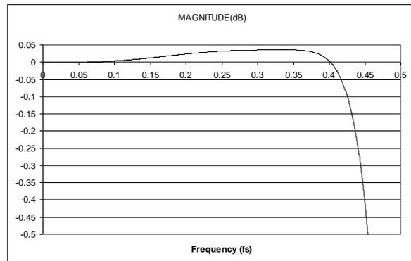
**Figure 43 DAC Digital Filter Ripple (Sloping Stopband Mode)**
