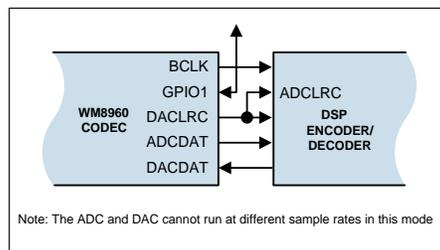
**Figure 24 Master Mode with ADCLRC as GPIO**
