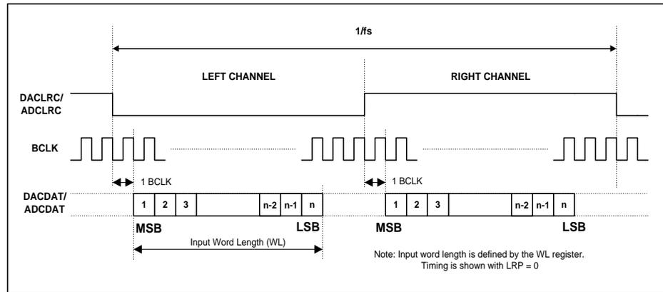
**Figure 28 I<sup>2</sup>S Justified Audio Interface (assuming n-bit word length)**
