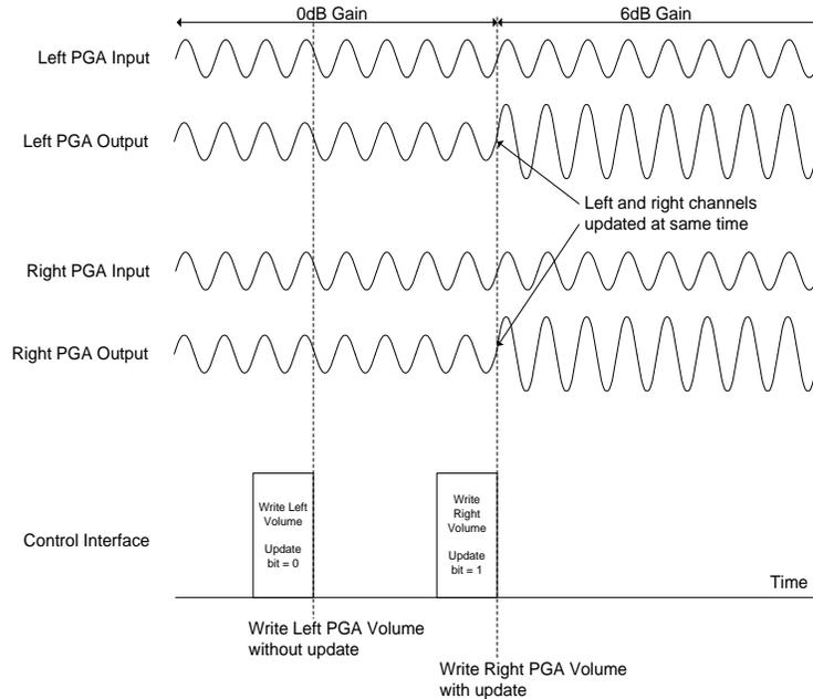
**Figure 16 Simultaneous Left and Right Volume Updates**
