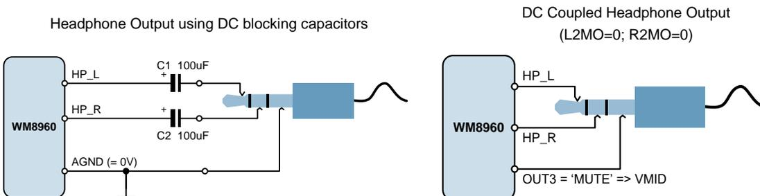
**Figure 15 Recommended Headphone Output Configurations**
