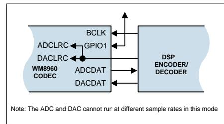
**Figure 25 Slave Mode with ADCLRC as GPIO**
