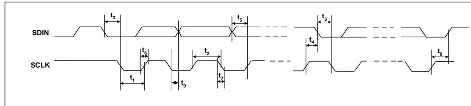
**Figure 4 Control Interface Timing – 2-Wire Serial Control Mode**
