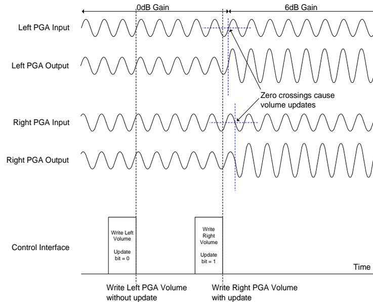
**Figure 18 Volume Update using Zero Cross Detection**
