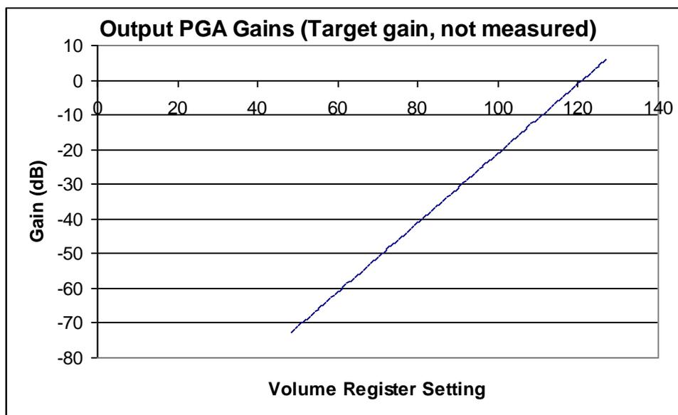
Figure 1 Output PGA Gains (LOUT1VOL, ROUT1VOL, SPKLVOL, SPKRVOL)
