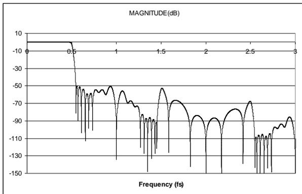
**Figure 40 DAC Digital Filter Frequency Response (Normal Mode)**
