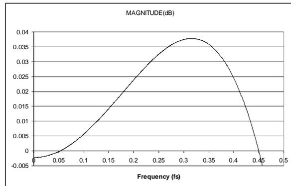
**Figure 41 DAC Digital Filter Ripple (Normal Mode)**
