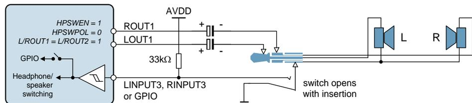
**Figure 20 Example Headset Detection Circuit Using Normally-Open Switch**
