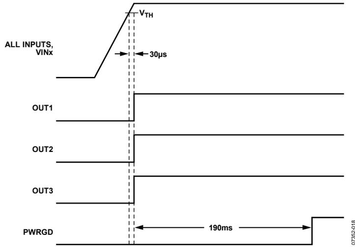
Figure 18. Power-Up Waveforms
