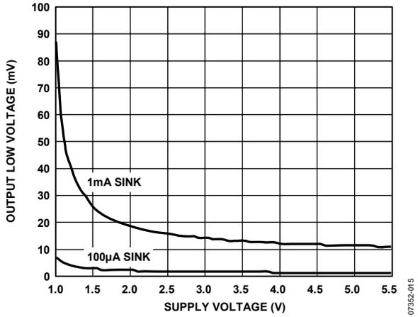
Figure 15. Output Low Voltage vs. Supply Voltage
