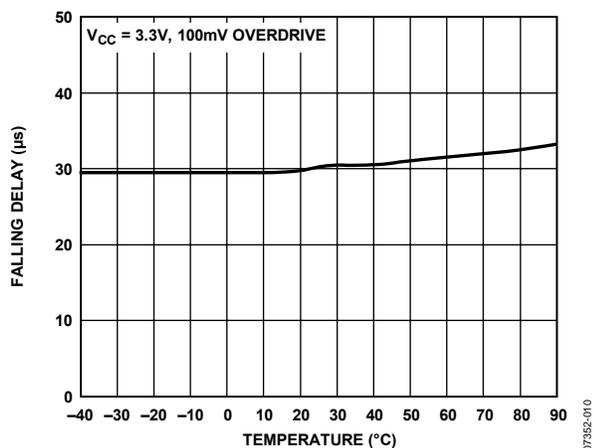
Figure 10. VINx to Output Falling Delay vs. Temperature
