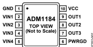
Figure 2. Pin Configuration
