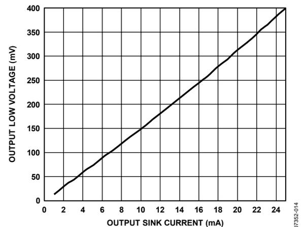
Figure 14. Output Low Voltage vs. Output Sink Current
