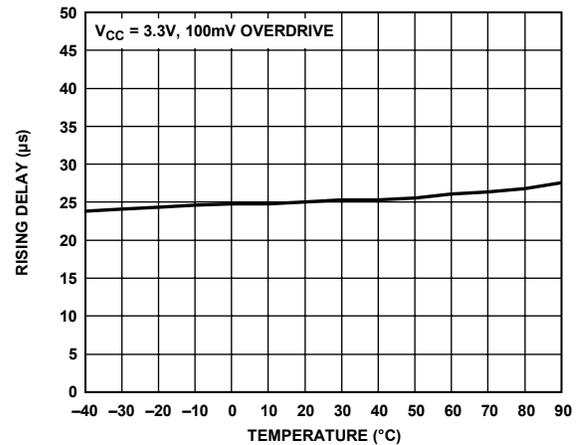
Figure 7. VIN1/VIN2/VIN3 to OUT1/OUT2/OUT3 Rising Delay vs. Temperature
