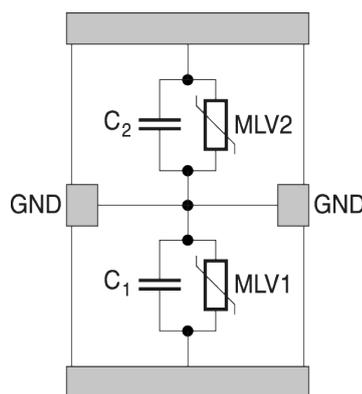
Model of EMI filtering with matched capacitances  $C_1$  and  $C_2$
