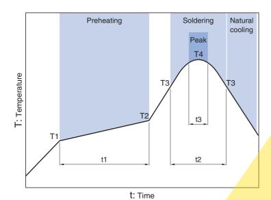
Soldering Preheating Peak Temp. Time Temp. Time Temp. Time T2 Т3 150°C 180°C 60 to 120s 230°C 250°C
