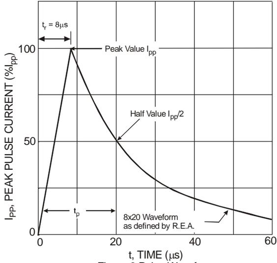
Figure 3 Pulse Waveform
