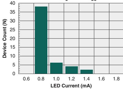
**Typical  $I_F$  for Switch Dropout**
