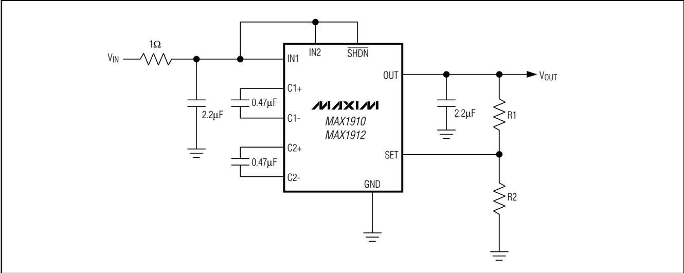
Figure 6. Output Voltage Set with a Resistor-Divider
