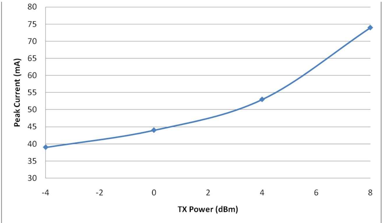
Figure 14: LE peak current vs. TX power
