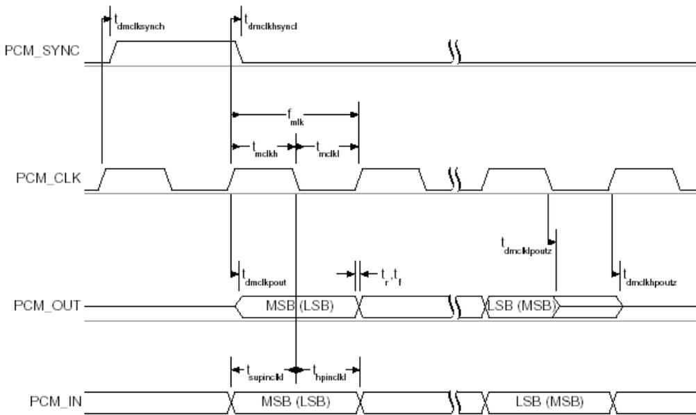
**Figure 24: PCM Master Timing Short Frame Sync**
