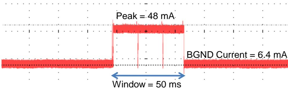
**Figure 11: LE scanning with 50 ms window**
