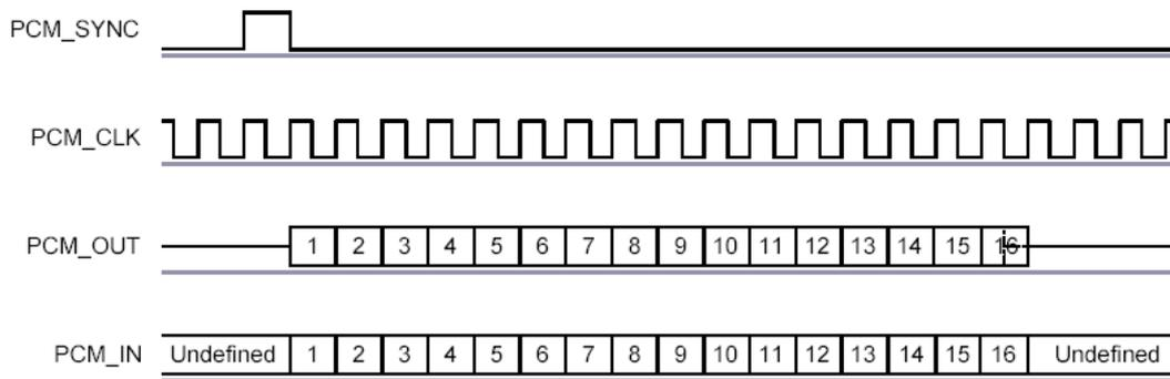
**Figure 19: Short Frame Sync (shown with 16-bit sample)**
