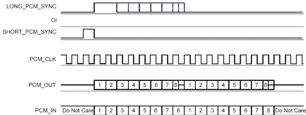
**Figure 20: Multi-slot Operation with 2 Slots and 8-bit Companded Samples**
