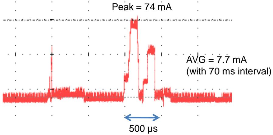
Figure 12: LE connected with 70 ms interval
