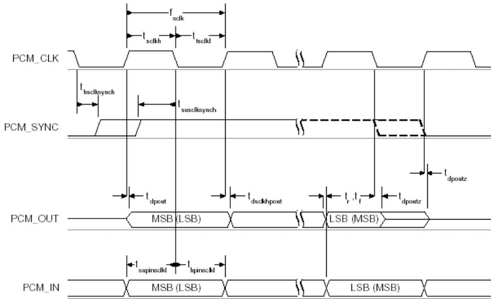
**Figure 25: PCM Slave Timing Long Frame Sync**
