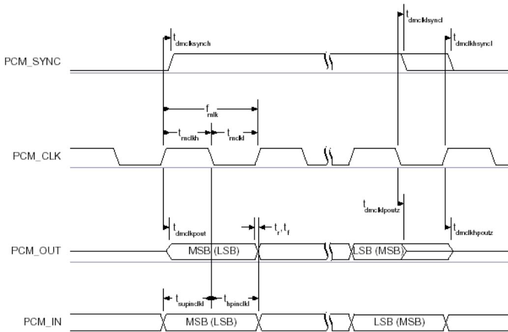
**Figure 23: PCM Master Timing Long Frame Sync**
