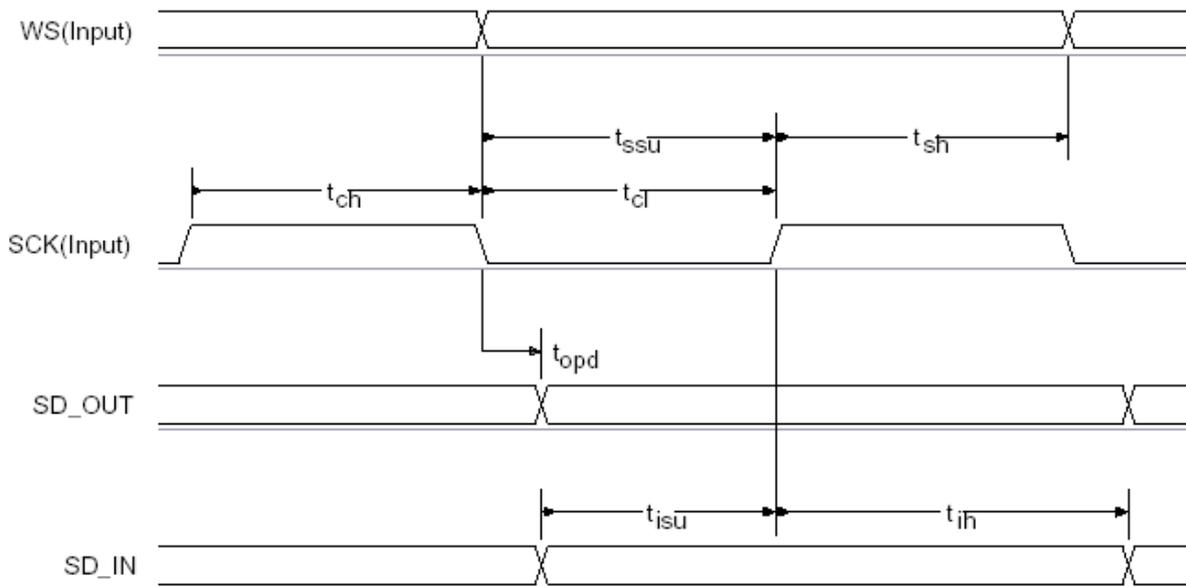
**Figure 28: Digital Audio Interface Slave Timing**
