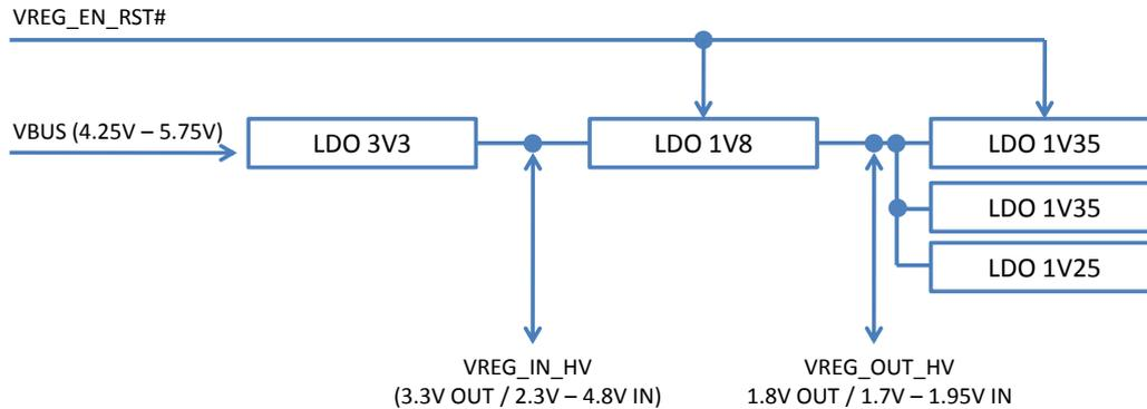
Figure 30: Internal regulators and powering of BT111
