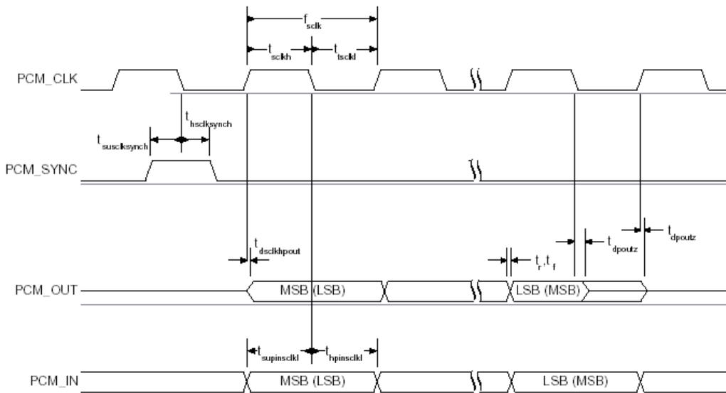
**Figure 26: PCM Slave Timing Short Frame Sync**
