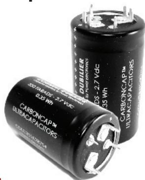
This leading edge, organic electrolyte D cell ultracapacitor can easily handle more than a half million duty cycles and has multiple pins and snap-in terminals for easy, reverse proof, robust, board mounting. They are suited for industrial power back up, renewable energy systems, short term UPS, and telecom applications.
