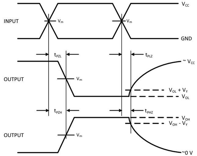
**Figure 4. Switching Waveforms**
