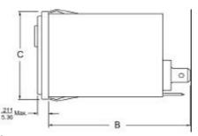
Mounting holes:  $\frac{.13}{3.3}$  Dia. (2) with .23 Dia. x 90° Counter sunk
