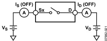
Figure 23. Off Leakage
