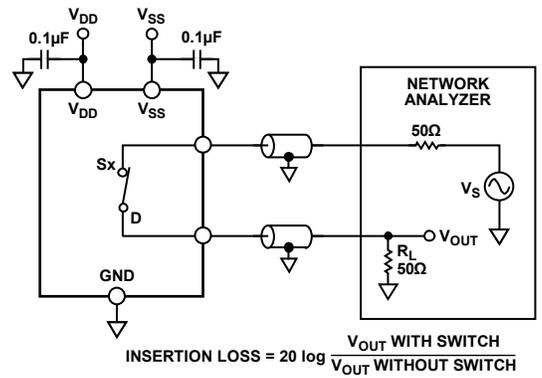
$$\text{INSERTION LOSS} = 20 \log \frac{V_{\text{OUT WITH SWITCH}}}{V_{\text{OUT WITHOUT SWITCH}}}$$
