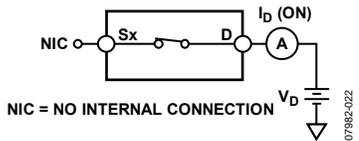
Figure 24. On Leakage
