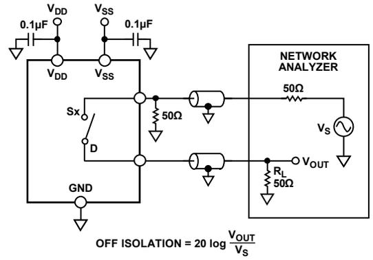
$$\text{OFF ISOLATION} = 20 \log \frac{V_{\text{OUT}}}{V_S}$$
