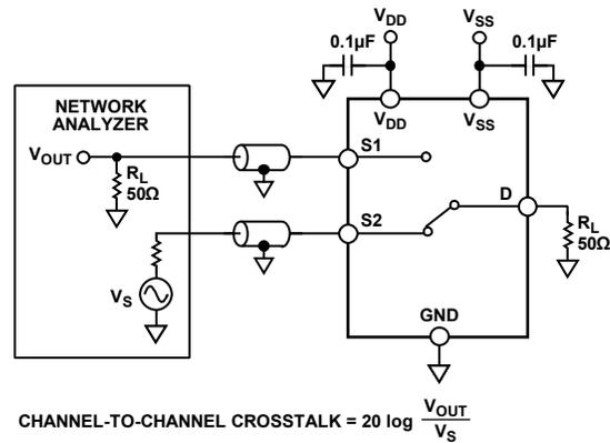
$$\text{CHANNEL-TO-CHANNEL CROSSTALK} = 20 \log \frac{V_{\text{OUT}}}{V_S}$$
