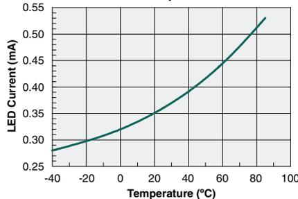
**Typical I<sub>F</sub> for Switch Dropout
