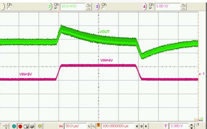
Figure 21. Line Transient,  $I_{LOAD}=1.0\text{ A}$ ,  $t_R=t_F=10\ \mu\text{s}$
