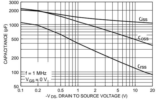
Figure 8. Capacitance Characteristics.
