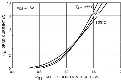
**Figure 5. Transfer Characteristics.**
