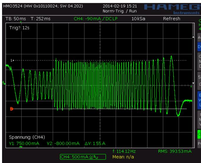
Figure 6.3 Scope shot: too small setting for  $PWM\_GRAD$
