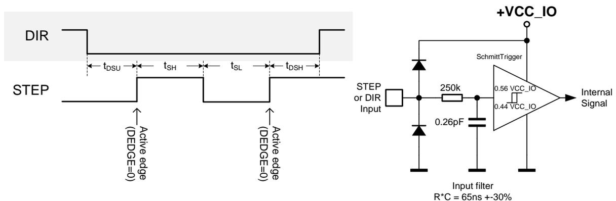
Figure 16.1 STEP and DIR timing, Input pin filter
