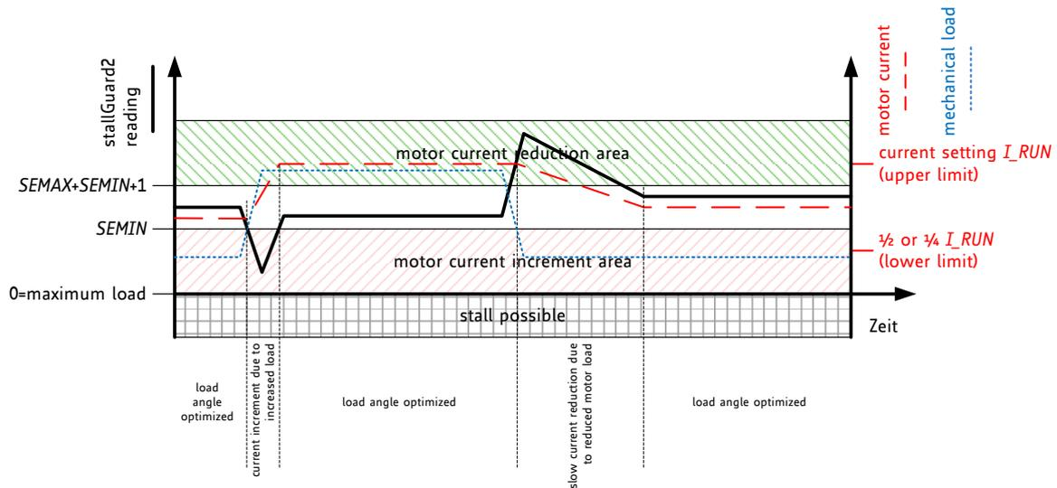
**Figure 15.1 CoolStep adapts motor current to the load**
