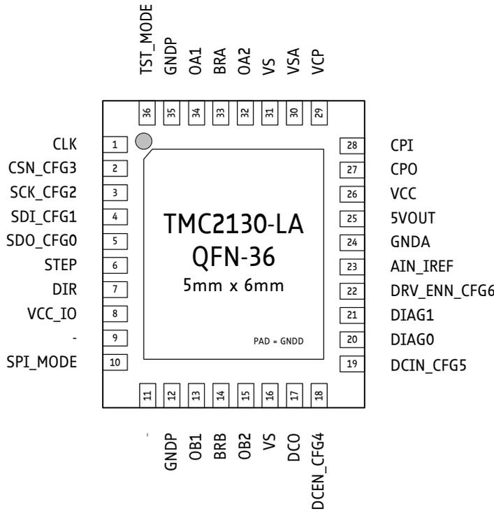
Figure 2.1 TMC2130-LA package and pinning QFN36 (5x6mm<sup>2</sup> body)
