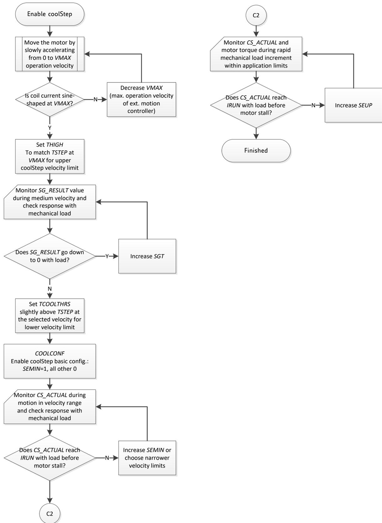
**Figure 22.3 Enabling CoolStep (only in combination with SpreadCycle)**
