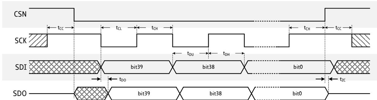
Figure 4.1 SPI timing
