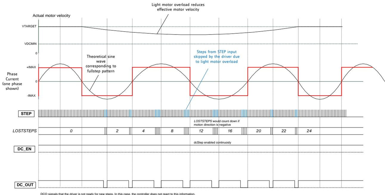
**Figure 18.3 Motor moving slower than STEP input due to light overload. LOSTSTEPS incremented**
