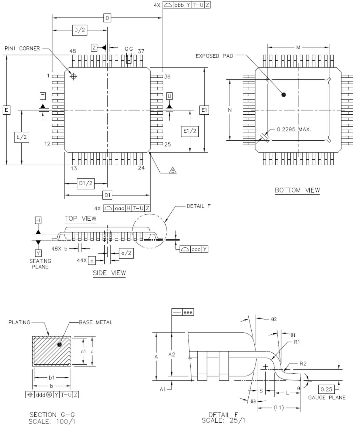
Figure 30.2 Dimensional drawings TQFP-EP48
