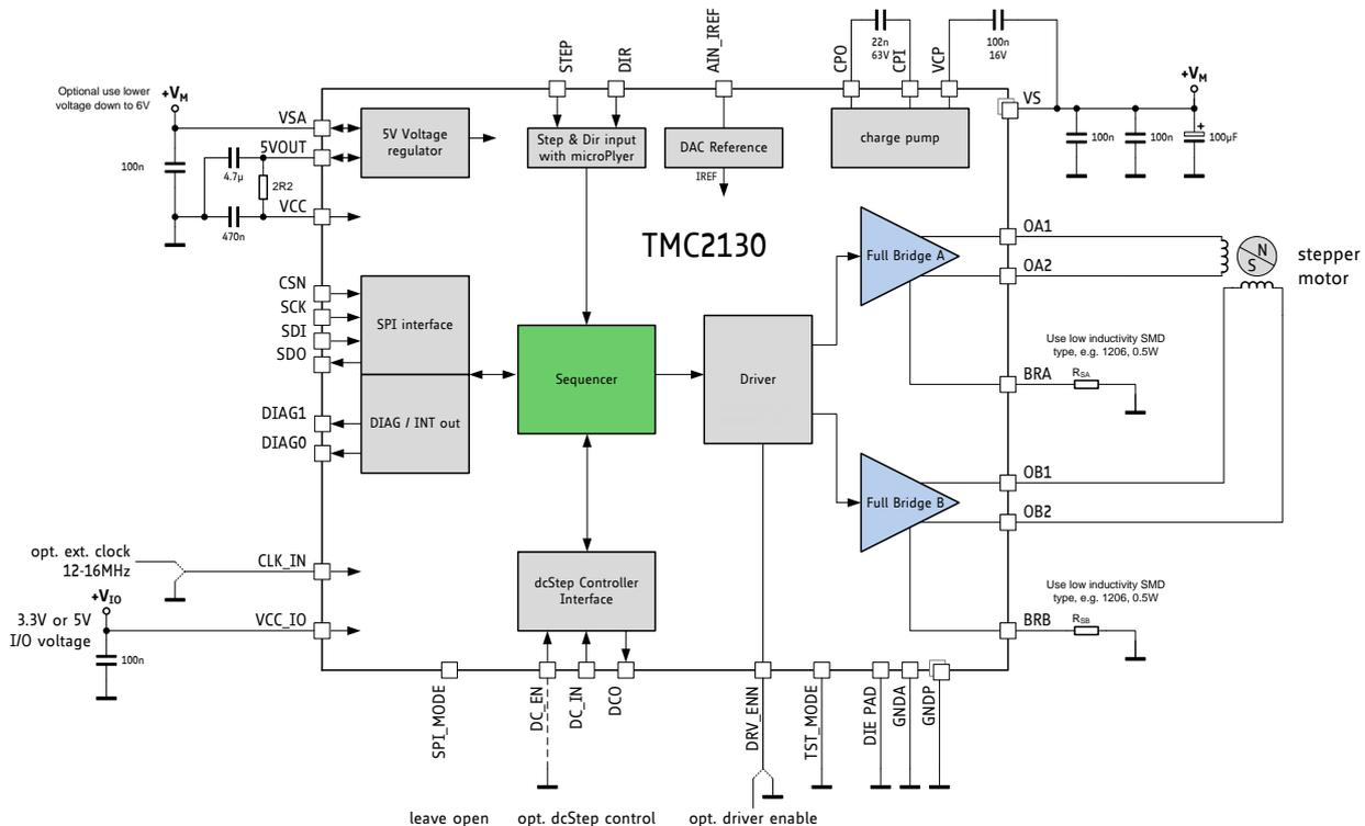
**Figure 3.1** Standard application circuit
