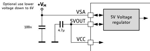
**Figure 3.2 Reduced number of filtering components**
