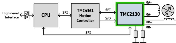
The CPU initializes the TMC4361A motion controller and the TMC2130. Thereafter, it sends target positions to the TMC4361. Now, the TMC4361 takes control over the TMC2130. Combining the TMC4361A and the TMC2130 offers diverse possibilities for demanding applications including servo drive features.
