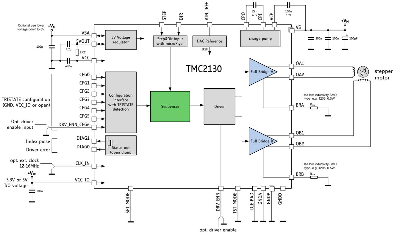
**Figure 24.1 Standalone operation with TMC2130 (pins shown with their standalone mode names)**
