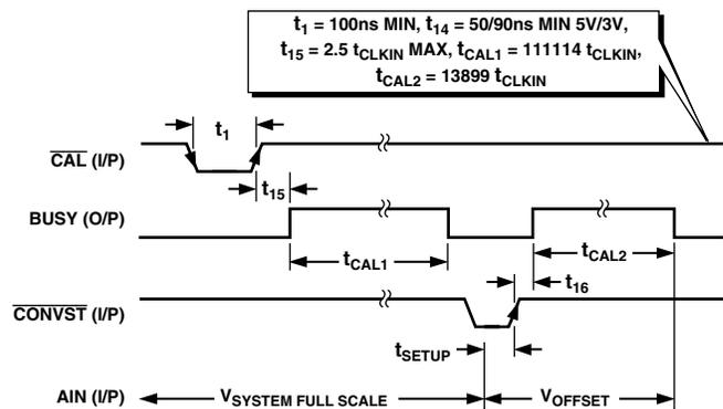
Figure 29. Timing Diagram for Full System Calibration
