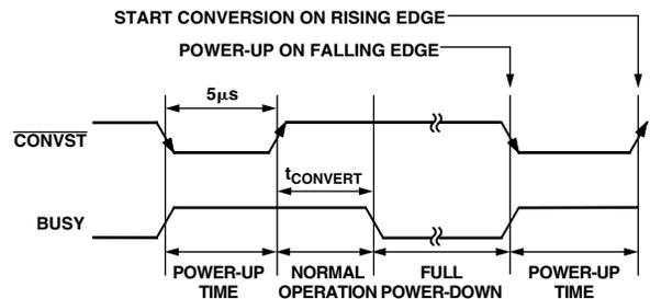
Figure 22. Power-Up Timing When Using CONVST Pin
