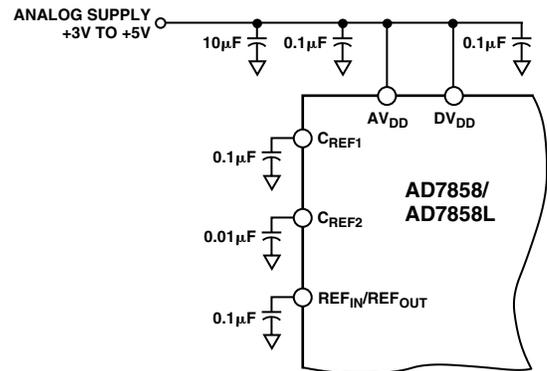
Figure 16. Relevant Connections When Using Internal Reference
