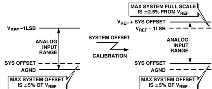
Figure 26. System Offset Calibration
