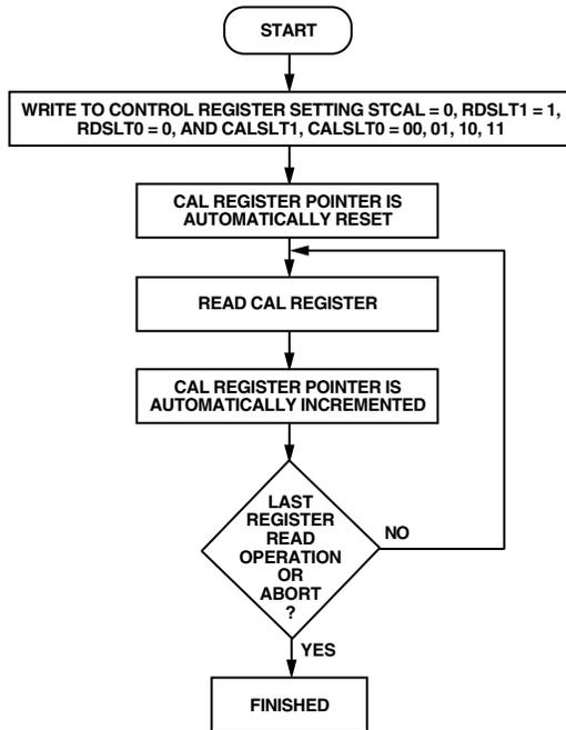
Figure 9. Flowchart for Reading from the Calibration Registers
