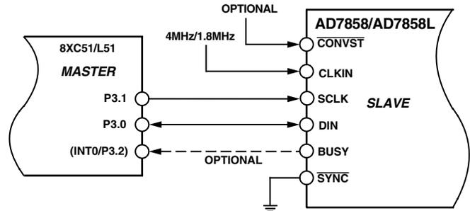
Figure 37. 8XC51/PIC16C42 Interface
