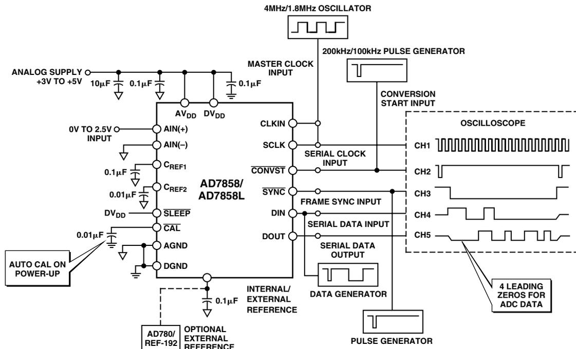
Figure 10. Typical Circuit
