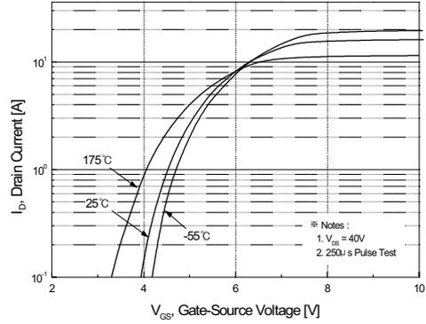
Figure 2. Transfer Characteristics
