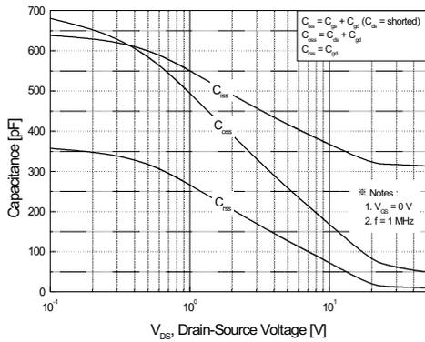
Figure 5. Capacitance Characteristics
