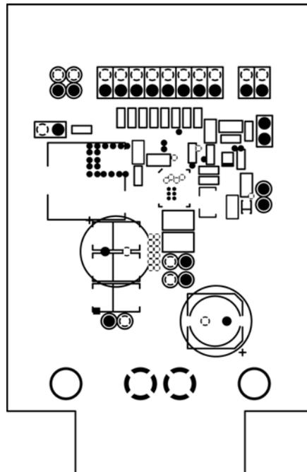
Figure 10. MIC26950 Evaluation Board Mid-Layer 1 (Ground Plane)
