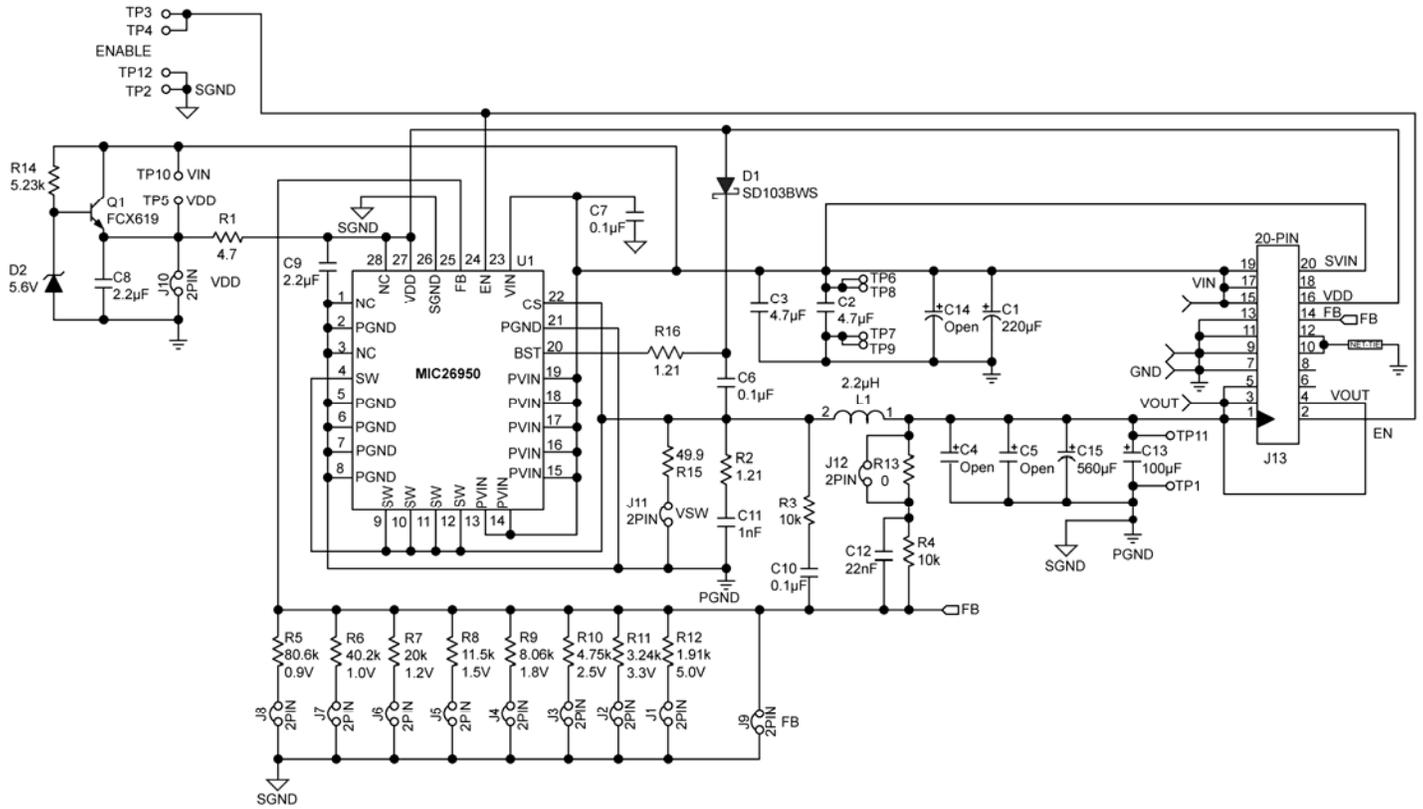
**Figure 8. Schematic of MIC26950 Evaluation Board**
