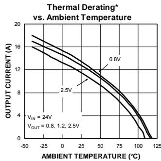
**Die Temperature\*** : The temperature measurement was taken at the hottest point on the MIC26950 case mounted on a 5 square inch 4 layer, 0.62", FR-4 PCB with 2oz finish copper weight per layer, see Thermal Measurement section. Actual results will depend upon the size of the PCB, ambient temperature and proximity to other heat emitting components.
