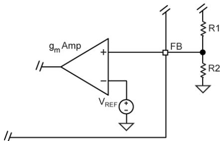
**Figure 6. Voltage-Divider Configuration**
