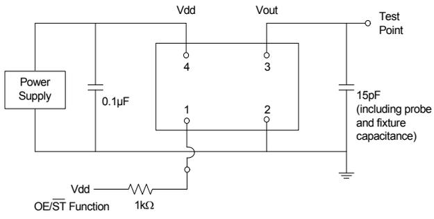
**Figure 2. Test Circuit**
