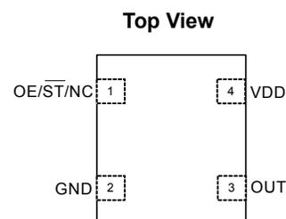
**Figure 1. Pin Assignments**
