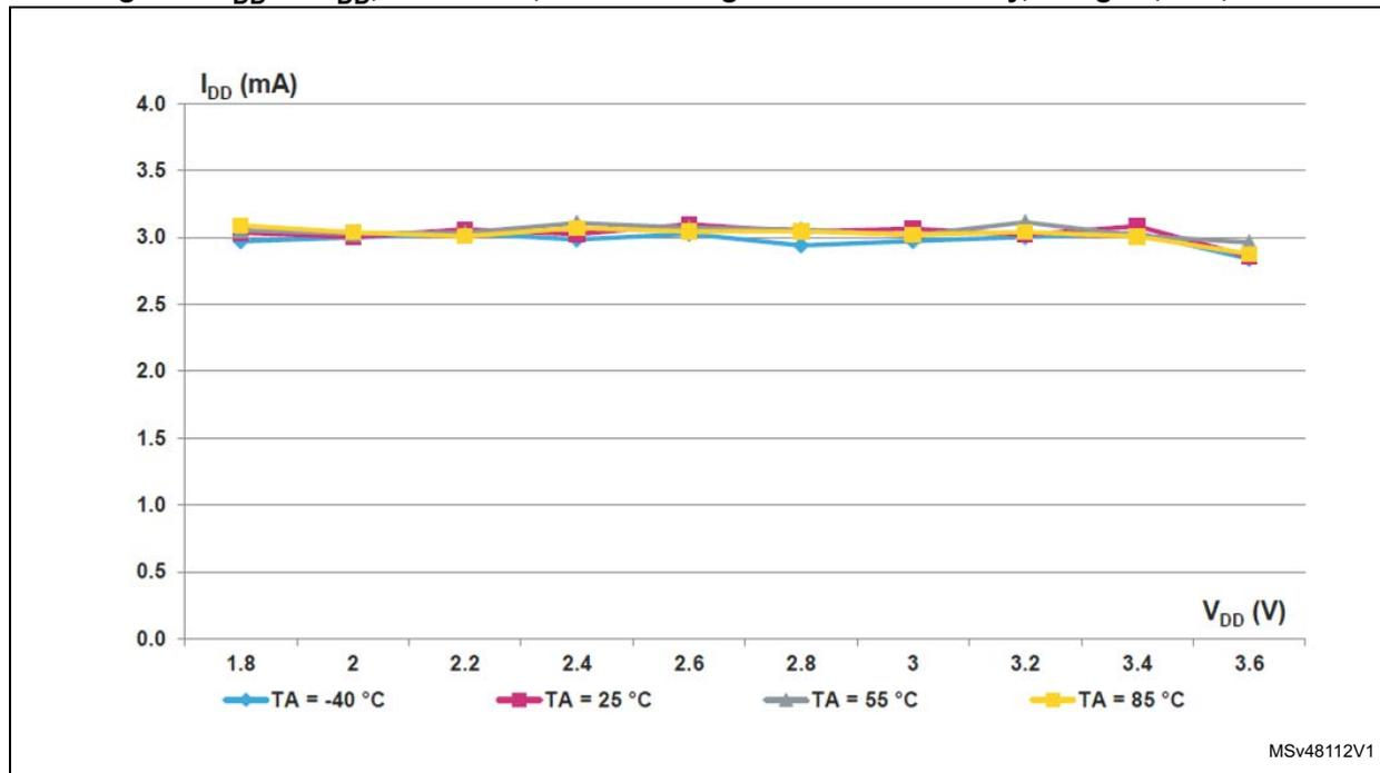
Figure 9. I<sub>DD</sub> vs V<sub>DD</sub>, Run mode, code running from Flash memory, Range 2, HSE bypass, 1 ws
