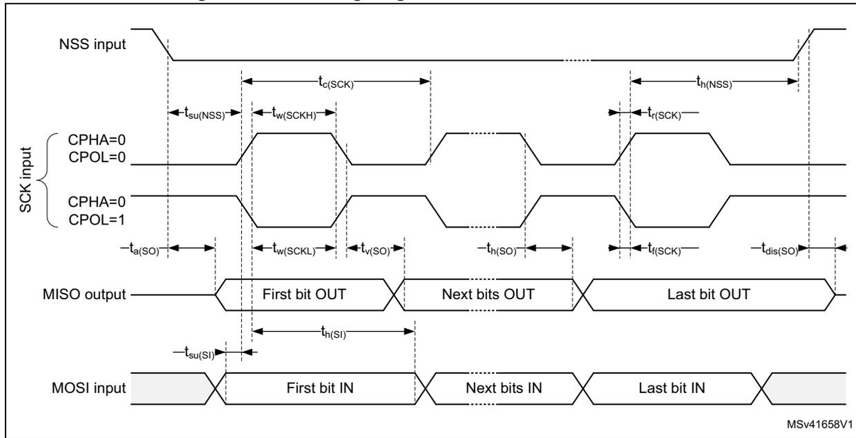
Figure 25. SPI timing diagram - slave mode and CPHA = 1<sup>(1)</sup>
