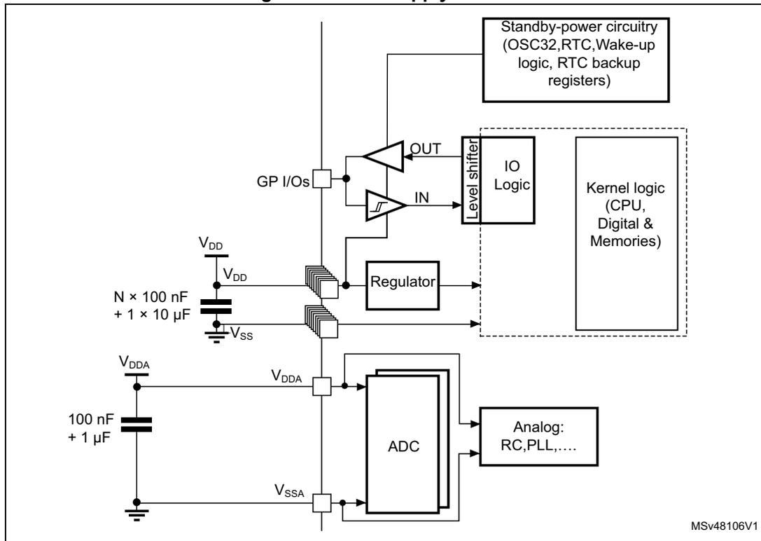
1. V<sub>SSA</sub> is internally connected to V<sub>SS</sub> on all packages.
