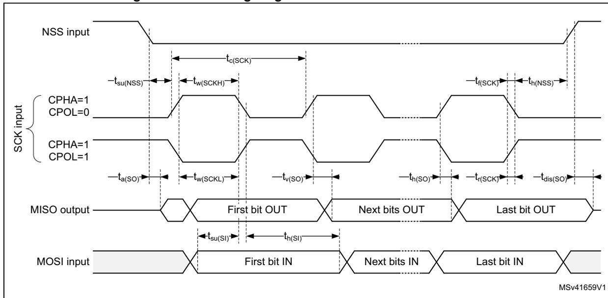
1. Measurement points are done at CMOS levels:  $0.3V_{DD}$  and  $0.7V_{DD}$ .
