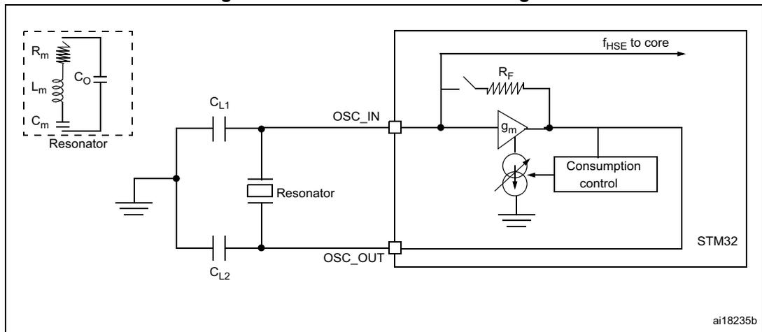
**Low-speed external clock generated from a crystal/ceramic resonator**
