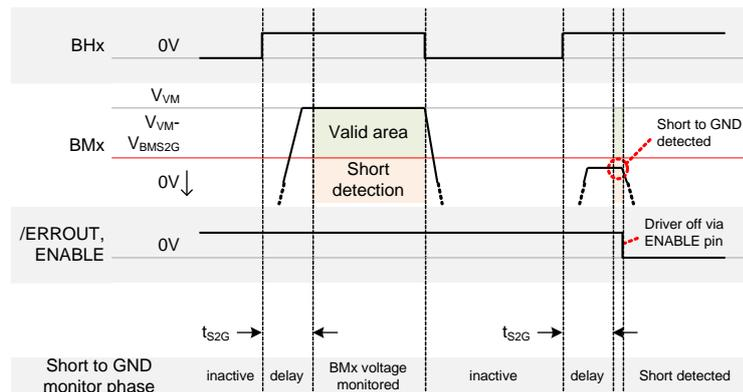
figure 12: timing of the short to GND detector
