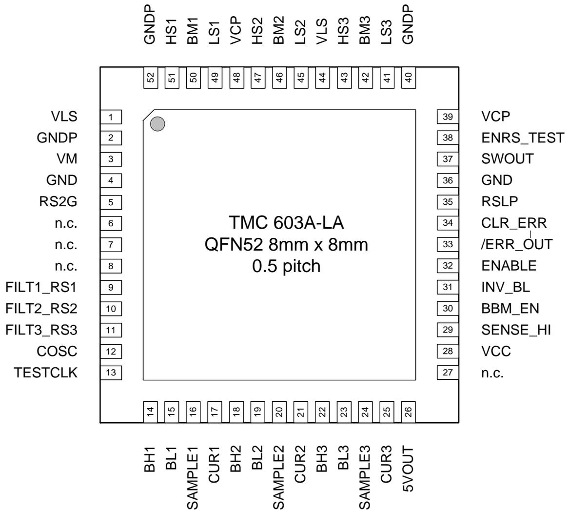
figure 2: pinning / QFN52 package (top view)
