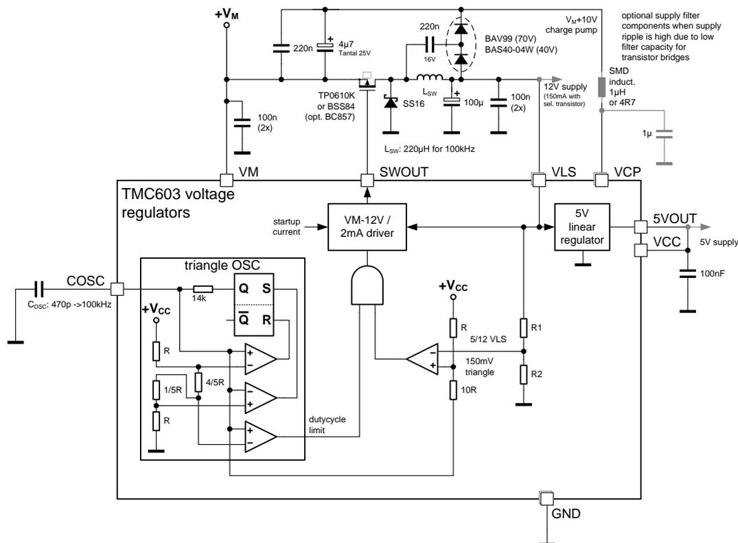
figure 16: power supply block with example values
