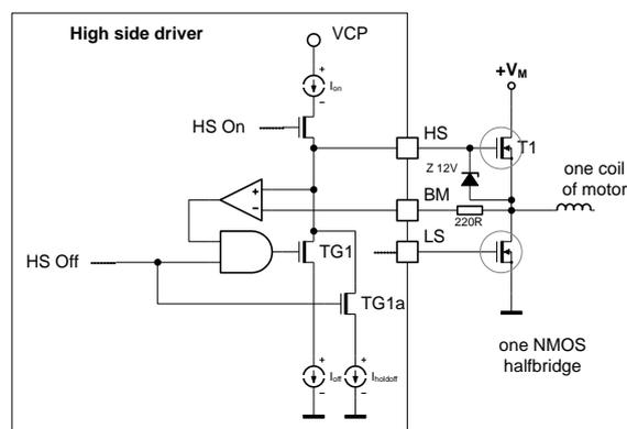
figure 5: principle of high-side driver (pat. fil.)
