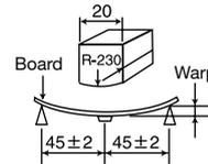
Capacitance measurement shall be conducted with the board bent (Unit: mm)
