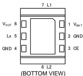
\* If the pad needs to be connected to other pins, it should be connected to the GND.
