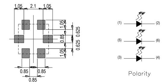
Note: Tolerances unless mentioned ±0.1mm. Unit = mm Suggested pad dimension is just for reference only. Please modify the pad dimension based on individual need.
