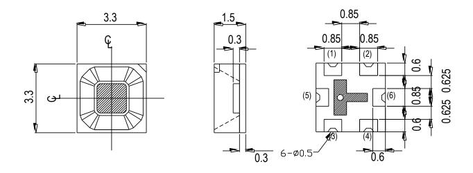
For Reflow Soldering(Propose)
