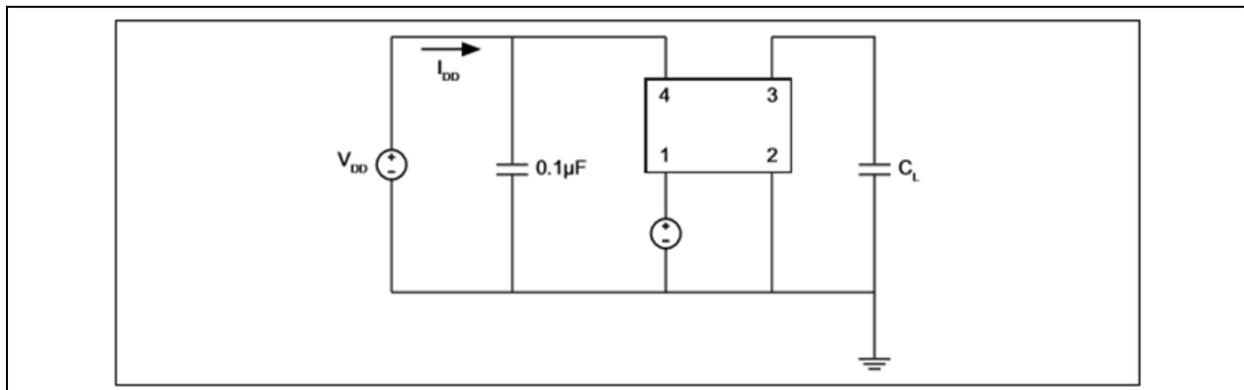
FIGURE 5-1: Test Circuit.
