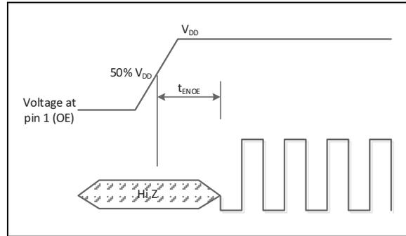
**FIGURE 6-3:** Enable Time with Pin 1 Configured as OE.
