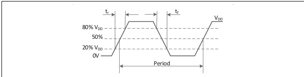
FIGURE 4-1: Output Waveform.
