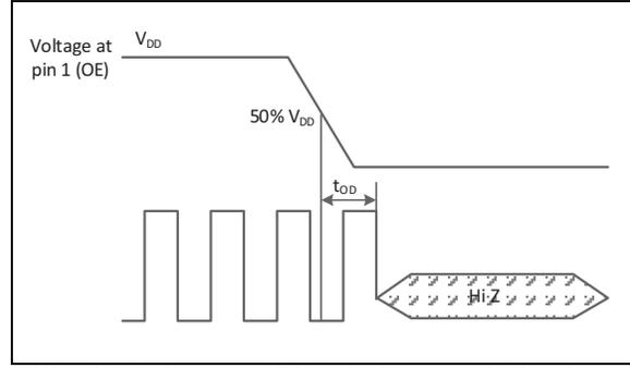
**FIGURE 6-4:** Disable Time with Pin 1 Configured as OE.
