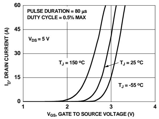
Figure 5. Transfer Characteristics
