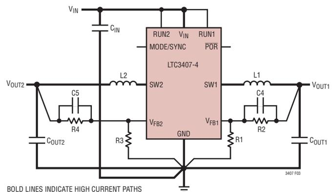
Figure 3. LTC3407-4 Layout Diagram (See Board Layout Checklist)
