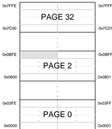
**Figure 20: Flash Address (in unified memory space)**
