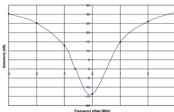
Figure 59: Typical Selectivity at 500 kBaud. IF Frequency is 307.4 kHz.
