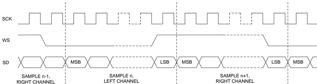
**Figure 42: I<sup>2</sup>S Digital Audio Signaling**
