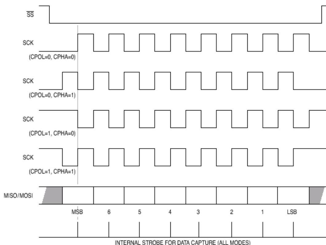
Figure 41: SPI Dataflow
