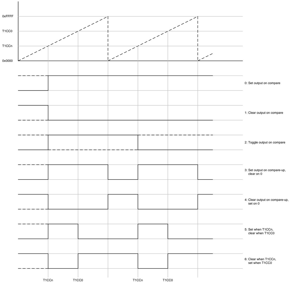
**Figure 32: Output Compare Modes, Timer Free-running Mode**
