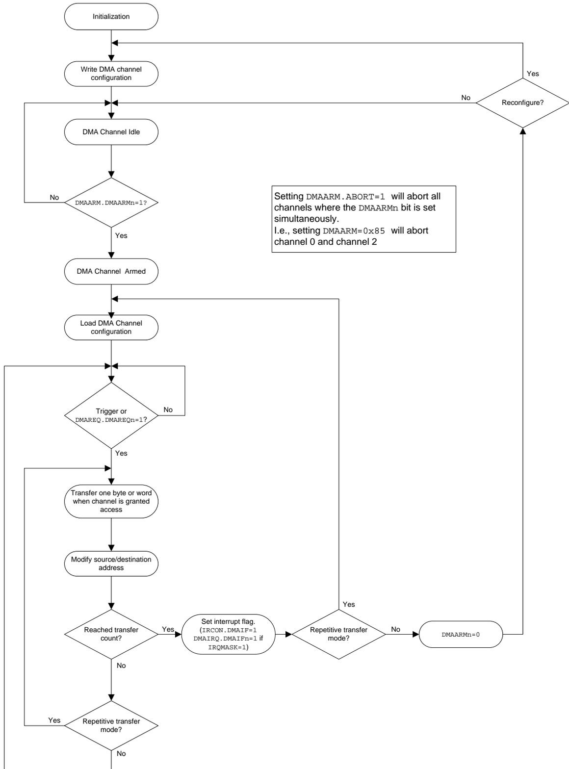
Figure 26: DMA Operation
