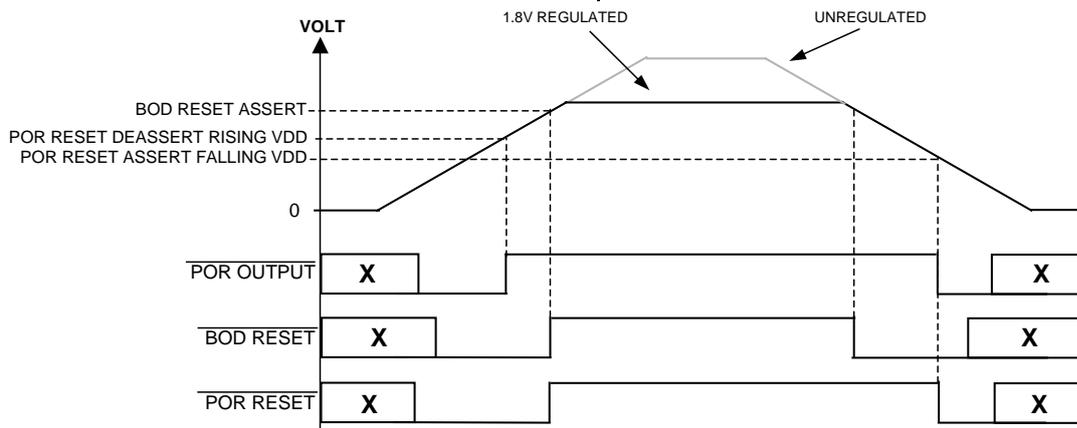
**Figure 19: Power-On-Reset and Brown Out Detector Operation**
