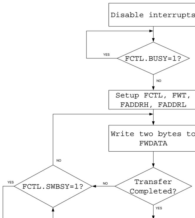
Figure 23: CPU Flash Write Executed from RAM
