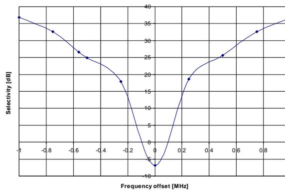
Figure 56: Typical Selectivity at 10 kBaud. IF Frequency is 273.9 kHz.
