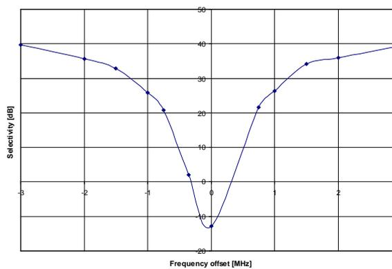
Figure 57: Typical Selectivity at 250 kBaud. IF Frequency is 177.7 kHz.
