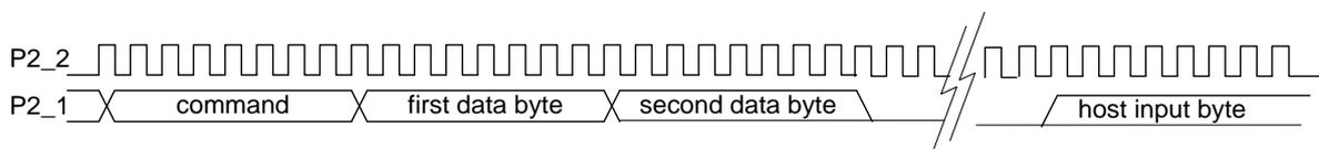
Figure 17: Debug Interface Timing Diagram
