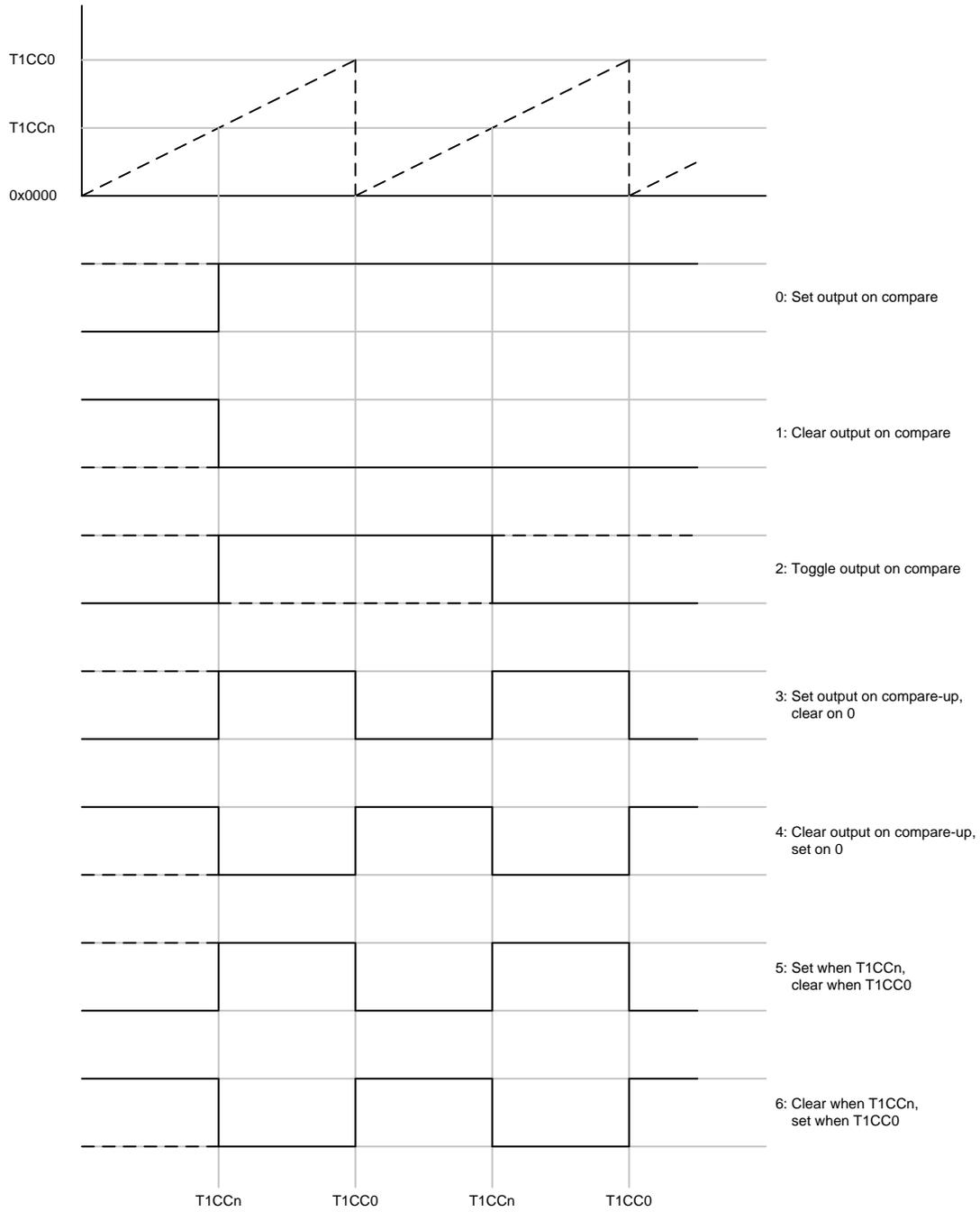
Figure 33: Output Compare Modes, Timer Modulo Mode
