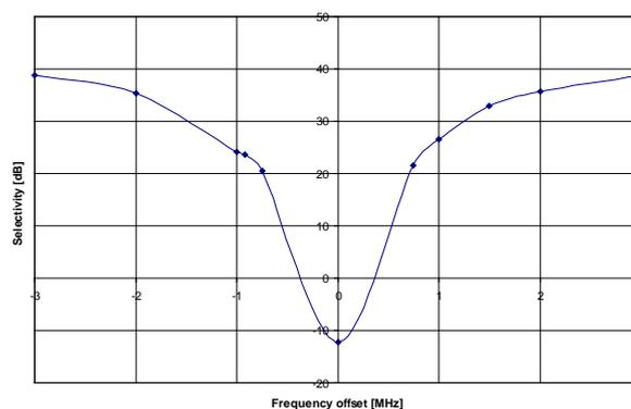
Figure 58: Typical Selectivity at 250 kBaud. IF Frequency is 457 kHz.
