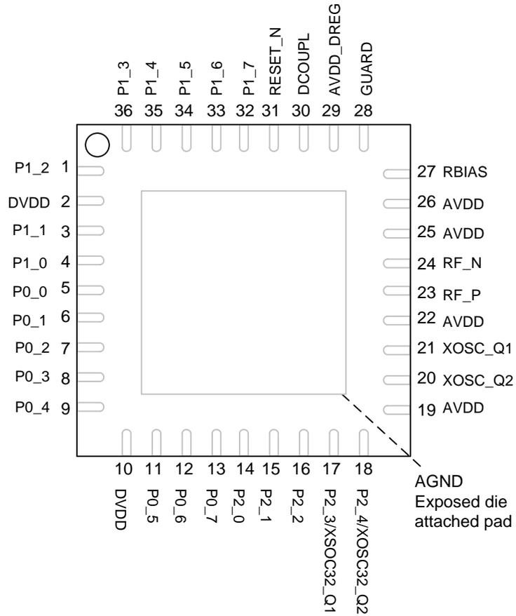
**Figure 7: CC2510Fx Pinout Top View**
