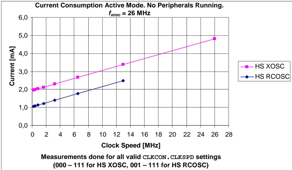
Figure 1: Current Consumption (Active Mode) vs. Clock Speed
