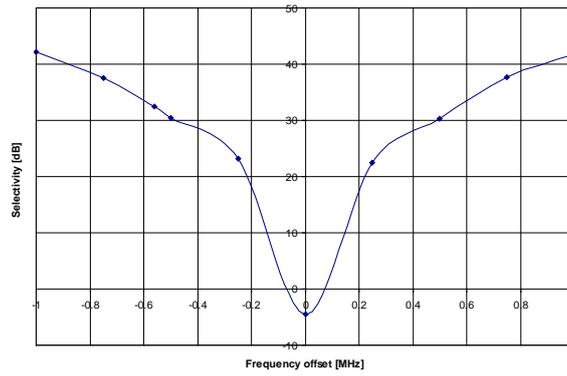
Figure 55: Typical Selectivity at 2.4 kBaud. IF Frequency is 273.9 kHz.
