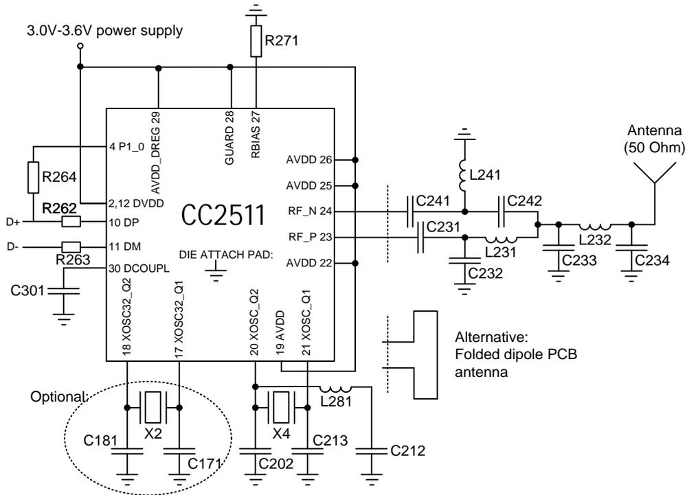
**Figure 12: Application Circuit for CC2511Fx with 3<sup>rd</sup> Overtone Crystal (excluding supply decoupling capacitors)**
