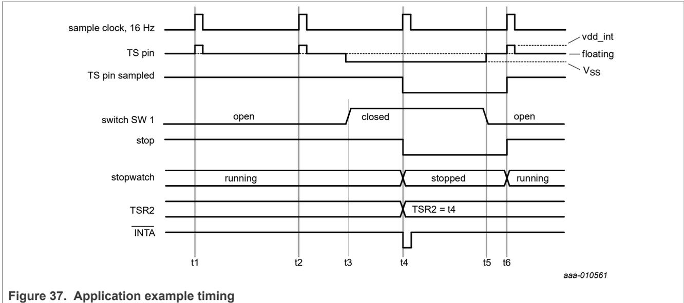
Figure 37. Application example timing
