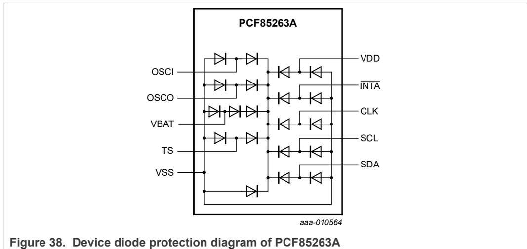
Figure 38. Device diode protection diagram of PCF85263A
