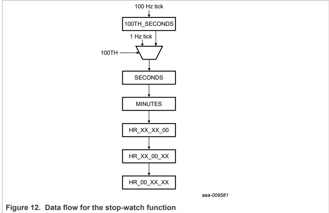
Figure 12. Data flow for the stop-watch function
