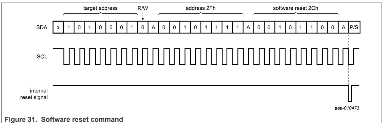
Figure 31. Software reset command
