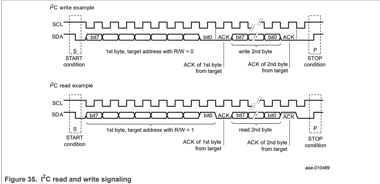
Figure 35. I<sup>2</sup>C read and write signaling
