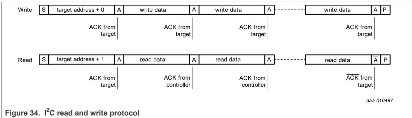
Figure 34. I<sup>2</sup>C read and write protocol
