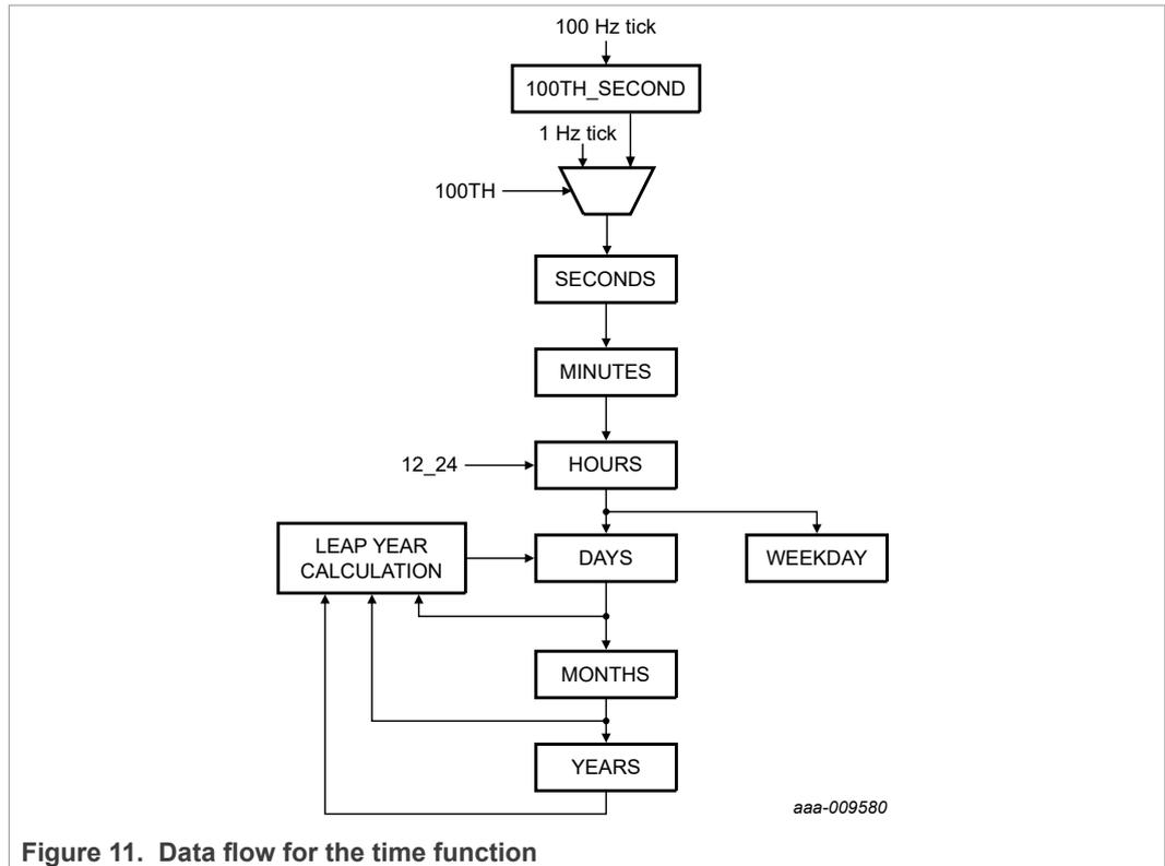
Figure 11. Data flow for the time function
