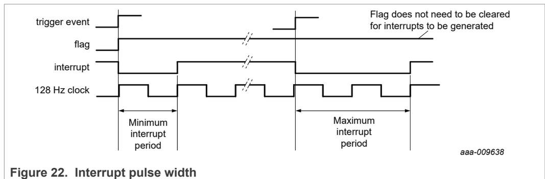
**Figure 22. Interrupt pulse width**
