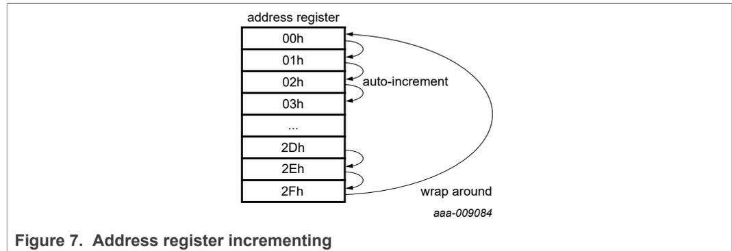
Figure 7. Address register incrementing
