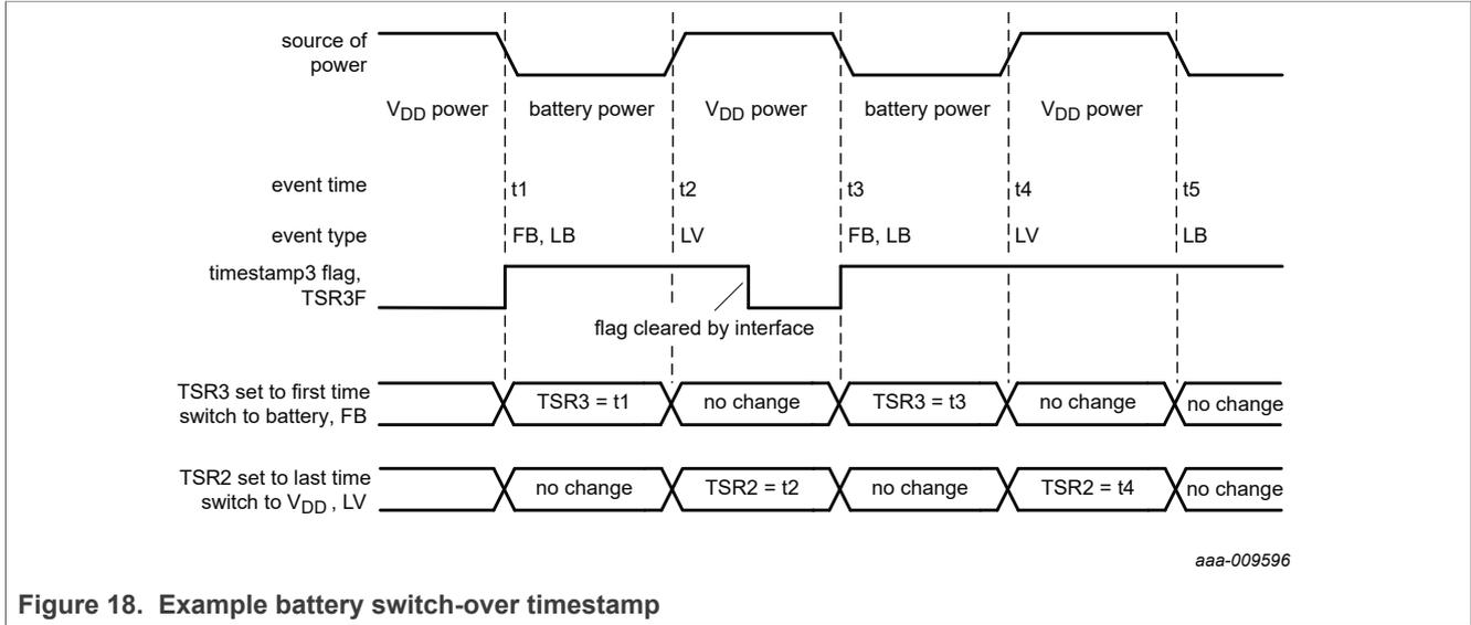
Figure 18. Example battery switch-over timestamp
