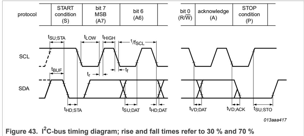
Figure 43. I<sup>2</sup>C-bus timing diagram; rise and fall times refer to 30 % and 70 %
