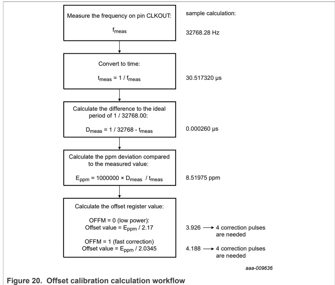
Figure 20. Offset calibration calculation workflow
