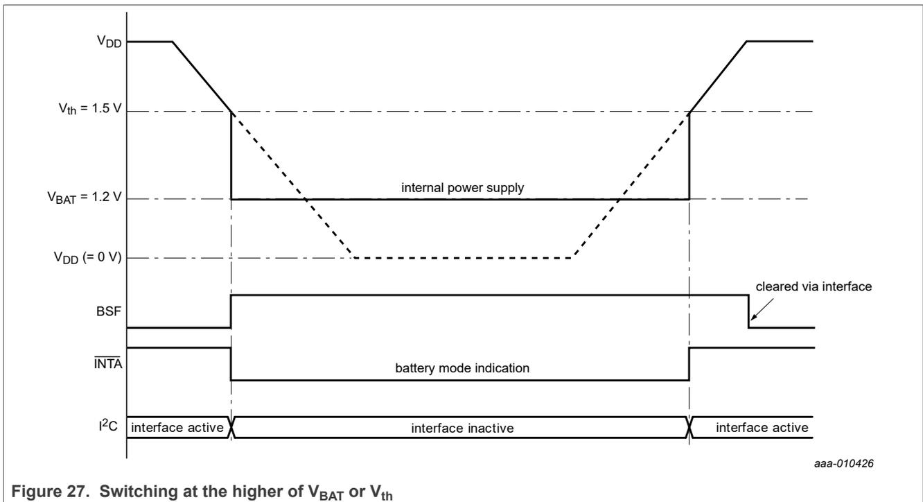
Figure 27. Switching at the higher of V<sub>BAT</sub> or V<sub>th</sub>
