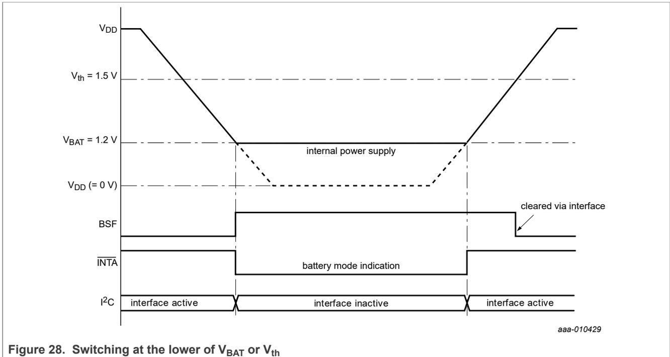
Figure 28. Switching at the lower of V<sub>BAT</sub> or V<sub>th</sub>
