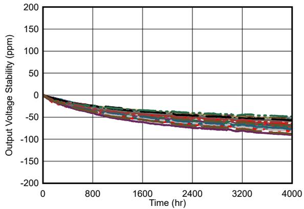
**Figure 7-25. Long-Term Stability LCCC package (First 4000 Hours)**
