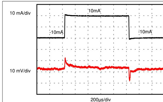
Figure 7-13. Load Transient Response ( $C_L = 10\ \mu\text{F}$ )
