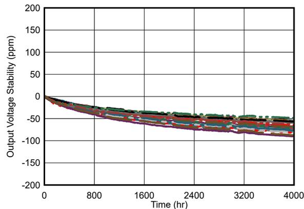
**Figure 8-4. Long Term Stability LCCC -4000 hours ( $V_{OUT}$ )**
