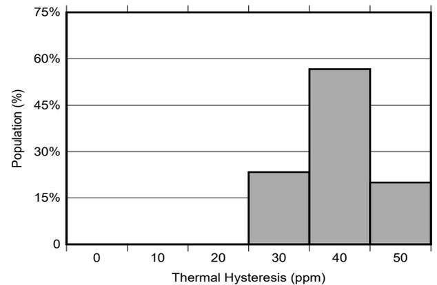
**Figure 7-24. REF7012QDGKR Thermal Hysteresis Distribution (0°C to 70°C)**
