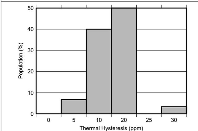
**Figure 7-23. REF7012QFKHR Thermal Hysteresis Distribution (0°C to 70°C)**
