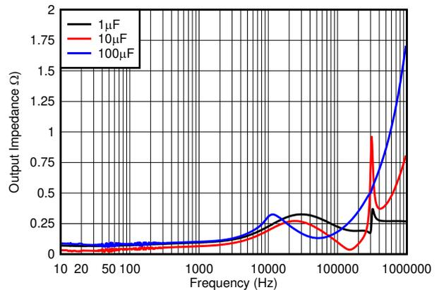
Figure 7-14. Output Impedance
