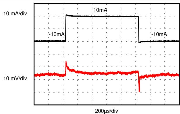
Figure 7-12. Load Transient Response ( $C_L = 1\ \mu\text{F}$ )
