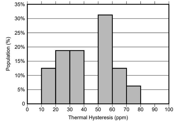
**Figure 7-22. REF7025QFKHR Thermal Hysteresis Distribution (0°C to 70°C)**
