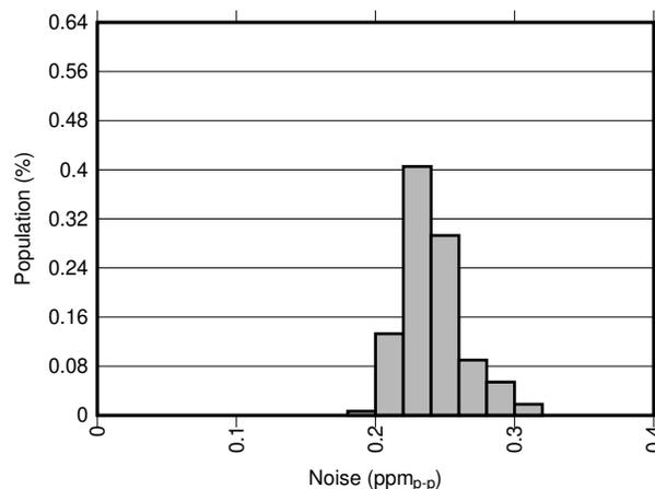
**Figure 8-10. 0.1-Hz to 10-Hz Voltage Noise Distribution**
