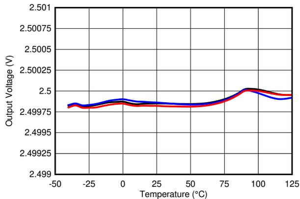
**Figure 7-1. Output Voltage Vs Free-Air Temperature (REF7025QFKHR)**
