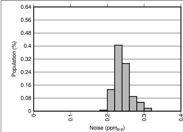
**Figure 7-19. 0.1-Hz to 10-Hz Voltage Noise Distribution (300 units)**
