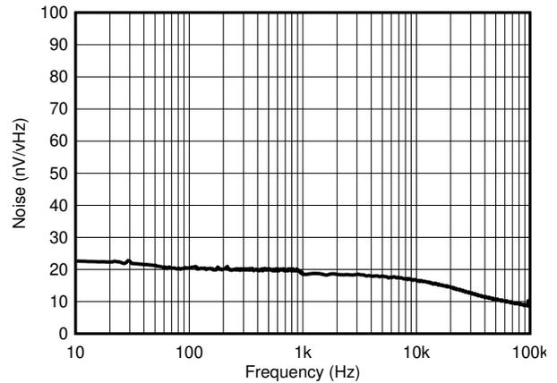
**Figure 7-20. Noise Performance 10 Hz to 100 kHz**
