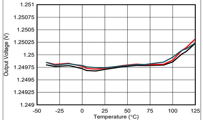
**Figure 7-2. Output Voltage Vs Free-Air Temperature (REF7012QDGKR)**
