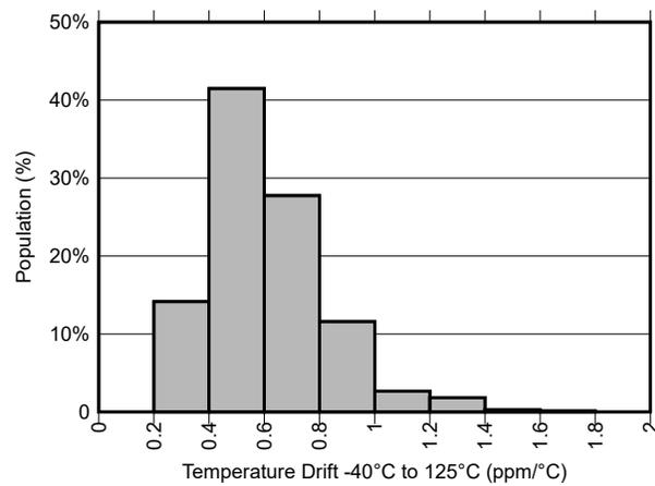
**Figure 7-3. Temperature Drift Distribution (REF7025QFKHR)**
