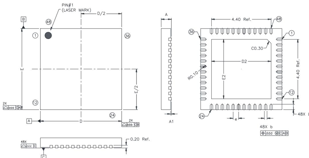
Figure 6. 48-Pin Quad Flat No Lead (QFN) Package
