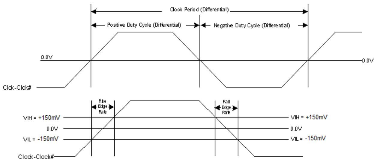
**Figure 4. Differential Output Signals (for AC Parameters Measurement)**
