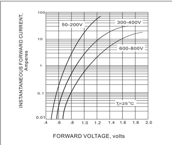
Fig.3 FORWARD CHARACTERISTICS
