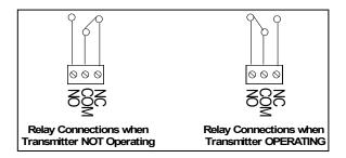
Relay output '1' provides a longer momentary output (approx ½ second) this may be removed (see below). For solenoid driven traps.
