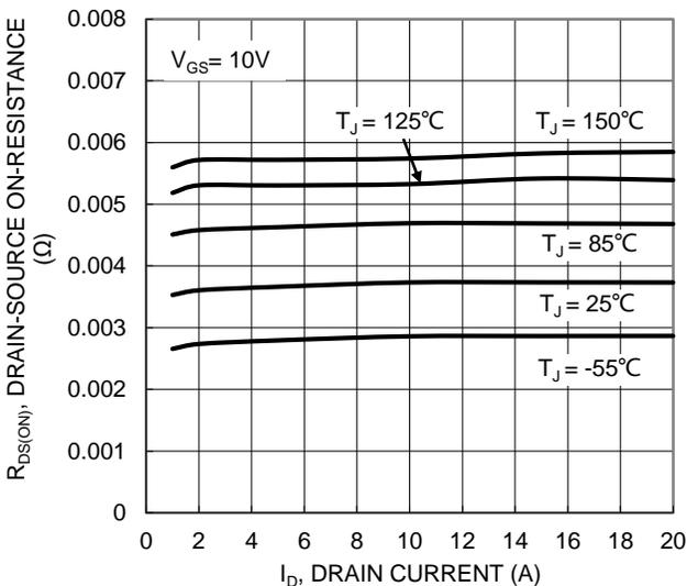
Figure 5. Typical On-Resistance vs. Drain Current and Temperature
