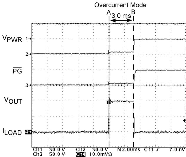
**Figure 9. Overcurrent Mode for More Than 3.0 ms**
