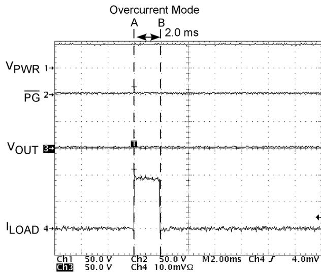
**Figure 10. Overcurrent Mode for Less Than 3.0 ms**
