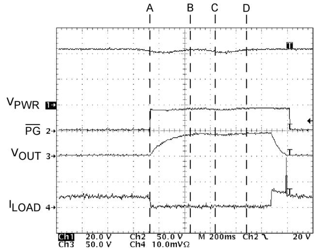
**Figure 15. Start-Up Timer Protection Against Undervoltage Faults**
