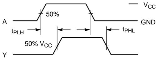
Figure 3. Switching Waveforms
