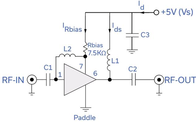
Fig 3. Recommended Application Circuit
