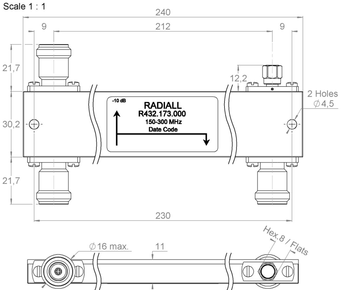
All dimensions are in mm. Tolerances according ISO 2768 m-H
