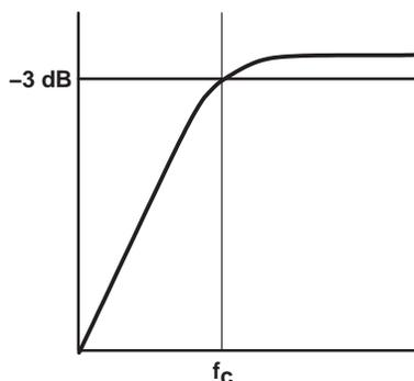
$$f_{c(\text{high})} = \frac{1}{2\pi R_L C_C} \quad (13)$$
