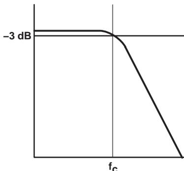
$$f_{c(\text{lowpass})} = \frac{1}{2\pi R_F C_F} \quad (7)$$
