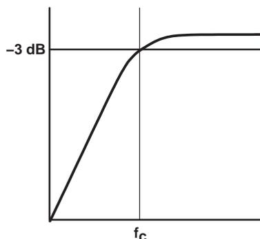
$$f_{c(\text{highpass})} = \frac{1}{2\pi R_I C_I} \quad (8)$$
