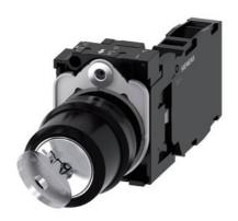
RONIS key-operated switch, 22 mm, round, plastic, lock number SB30, with 2 keys, 2 switch positions O-I, latching, 10:30h/13:30h, key removal O+I, with holder, 1 NO+1 NC, screw terminal, possible special locks: SB31, 421, 455, with laser labeling, upper case
