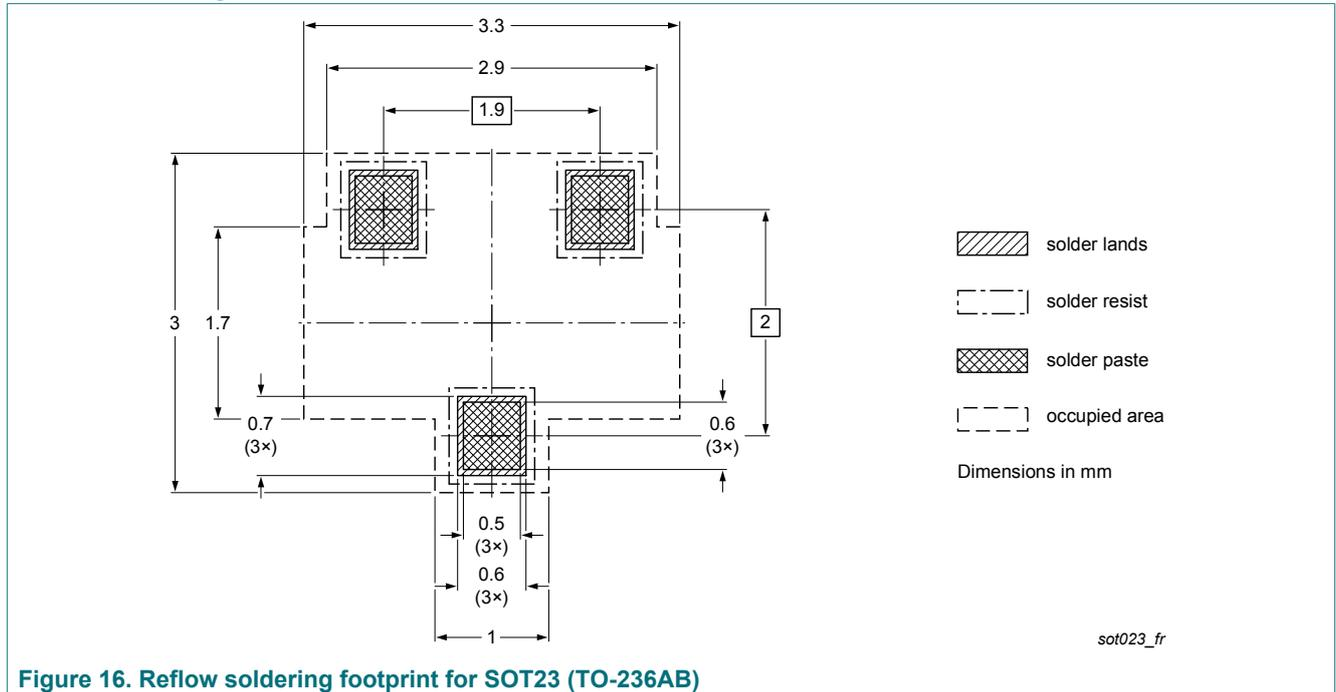
Figure 16. Reflow soldering footprint for SOT23 (TO-236AB)
