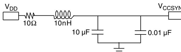
**Figure 4-2.**  $V_{CCSYN}$  Bypass
