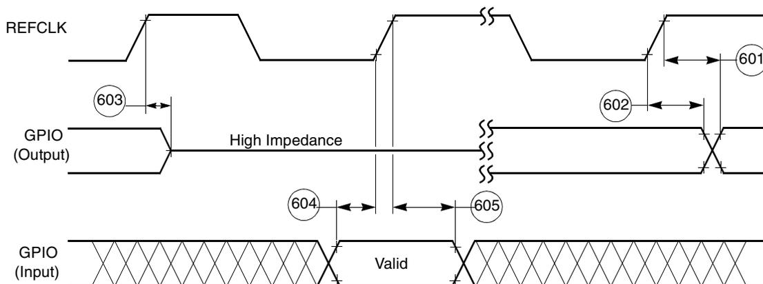
Figure 2-22. GPIO Timing
