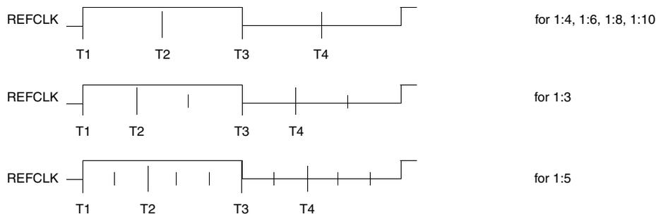
**Figure 2-5.** Internal Tick Spacing for Memory Controller Signals
