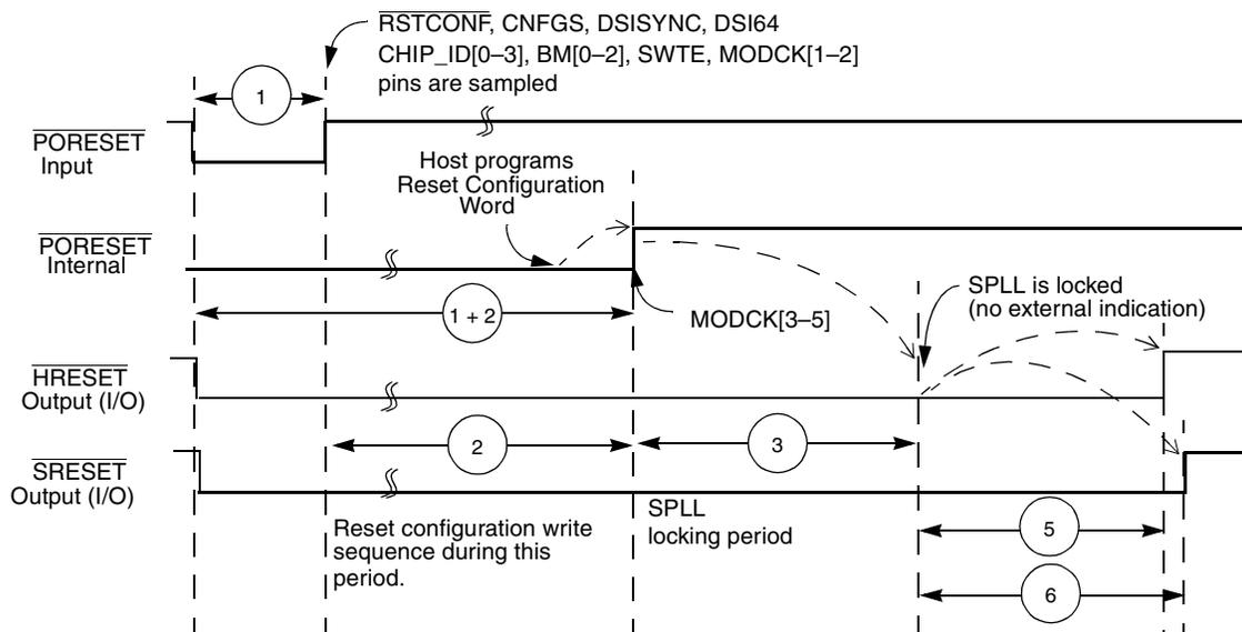
**Figure 2-4.** Timing Diagram for a Reset Configuration Write
