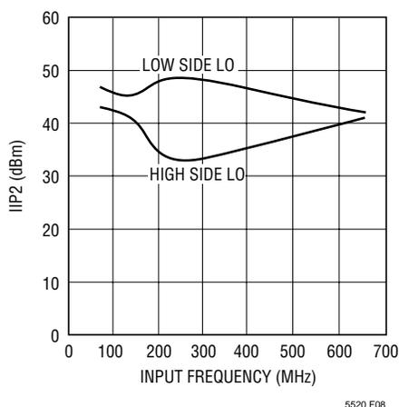
Figure 8. IIP2 vs Tuned IF Input Frequency
