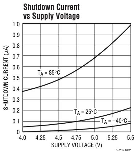
$V_{CC} = 5V_{DC}$ , EN = High,  $T_A = 25^\circ C$ , IF input =  $140MHz$  at  $-10dBm$ , LO input =  $1.76GHz$  at  $-5dBm$ , RF output measured at  $1900MHz$ , unless otherwise noted. For 2-tone inputs: 2nd IF input =  $141MHz$  at  $-10dBm$ . (Test Circuit Shown in Figure 2.)
